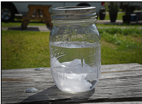
To determine each tissue's ability to break down, a single sheet of each brand was placed in a Mason jar with water and agitated. Dometic toilet paper (left) did not break down in the initial shake test, but after vigorous shaking the fibers started to come apart. It's important that when using this brand toilet paper, the holding tank is charged properly. Thetford's Aqua Soft (center) broke down immediately after the first few shakes. Company's Campa Soft, sold in Walmart, was equally as effective. The clear winner in the breakdown contest was Thetford's 1 ply toilet paper (right). It doesn't take much moisture for this paper to dissolve.
