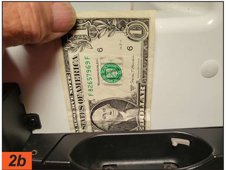
2a 2b The magnetic door gaskets (seal) must be tight to prevent the leakage of cold air. Inspect these gaskets frequently, because replacements are typically not available without buying the whole door. Aftermarket seals are usually not that effective. One simple way to determine if the gaskets are holding is to insert a dollar bill between door and refrigerator frame. There should only be a small amount of resistance when pulling the dollar bill out.
