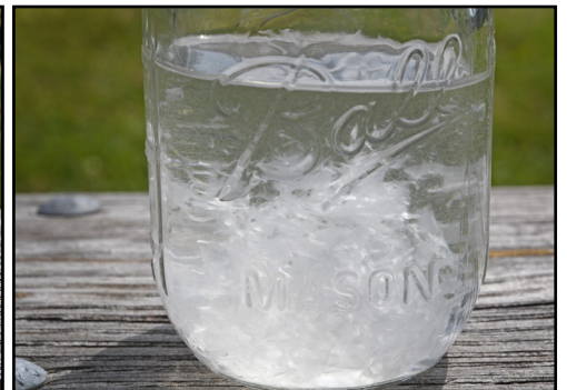
To determine each tissue's ability to break down, a single sheet of each brand was placed in a Mason jar with water and agitated. Dometic toilet paper (left) did not break down in the initial shake test, but after vigorous shaking the fibers started to come apart. It's important that when using this brand toilet paper, the holding tank is charged properly. Thetford's Aqua Soft (center) broke down immediately after the first few shakes. Company's Campa Soft, sold in Walmart, was equally as effective. The clear winner in the breakdown contest was Thetford's 1 ply toilet paper (right). It doesn't take much moisture for this paper to dissolve.
