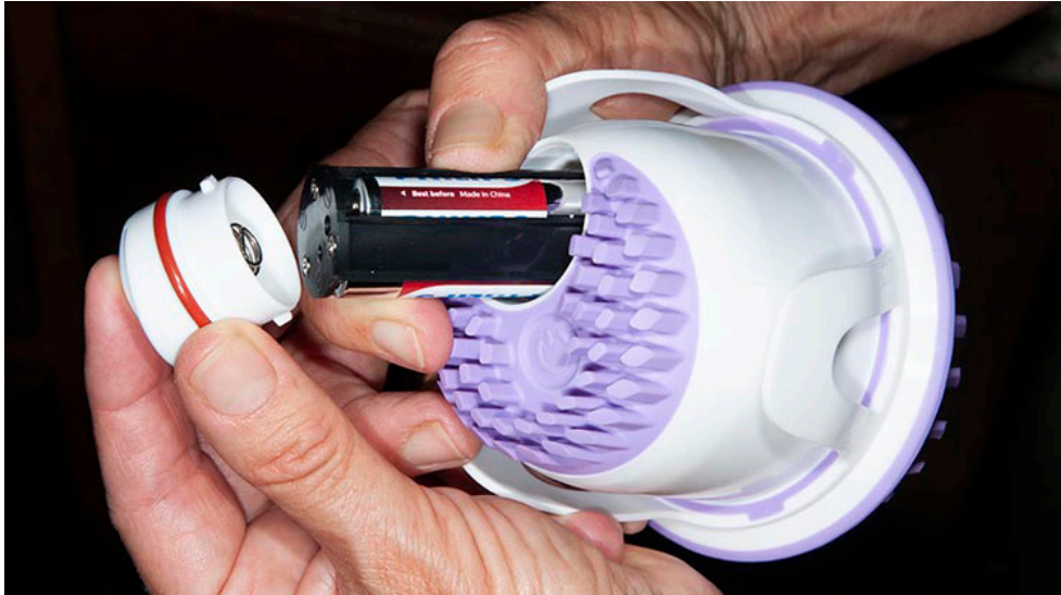
The motor that creates the vibrations operates on three AAA batteries, which are placed in a waterproof compartment.
