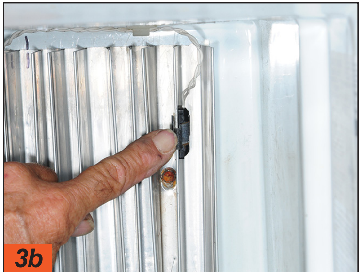
3a 3b A thermistor is used to communicate with the control board to set box temperatures. This sensor is mounted on the evaporator/cooling fins in the back of the refrigerator. Dometic mounts its thermistor on the first fin and can be moved up and down to adjust temperature, based on an adjacent instruction sticker. Norcold mounts its thermistor, which is fixed, on the third fin from the right. These thermistors can be tested for proper function by using an ohm meter (not shown) following the manufacturer's instructions, which are available online.
