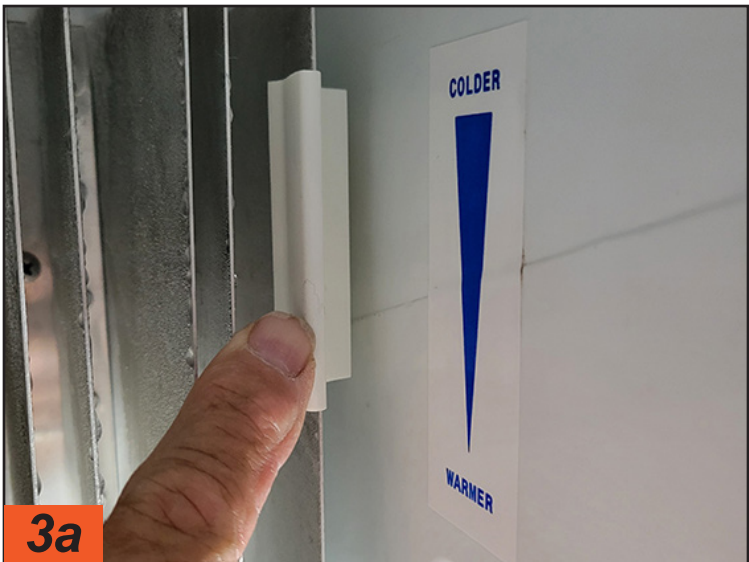
3a 3b A thermistor is used to communicate with the control board to set box temperatures. This sensor is mounted on the evaporator/cooling fins in the back of the refrigerator. Dometic mounts its thermistor on the first fin and can be moved up and down to adjust temperature, based on an adjacent instruction sticker. Norcold mounts its thermistor, which is fixed, on the third fin from the right. These thermistors can be tested for proper function by using an ohm meter (not shown) following the manufacturer's instructions, which are available online.
