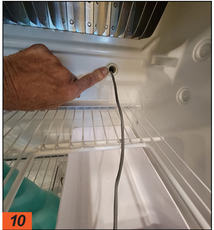
Power (12-volt DC) was routed through the condensation drain tube after temporarily removing the capture tray. Here both the positive and negative leads are routed because there is no logical place to get continuous power inside the box on Dometic refrigerators. The ground wire can be connected inside at the light fixture on Norcold models.
