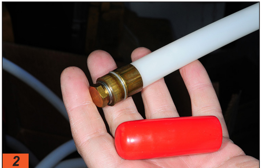
THIA by Proteng devices (tubes) are custom manufactured in the U.S.A. and are comprised of specialized materials and filled with clean agent gas (FM-200™). Brass fittings, protected by plastic covers, seal the contents in the devices. The system tubes are covered by a five-year warranty and should last up to 10 years, depending on where they are mounted. They are not user-serviceable.
