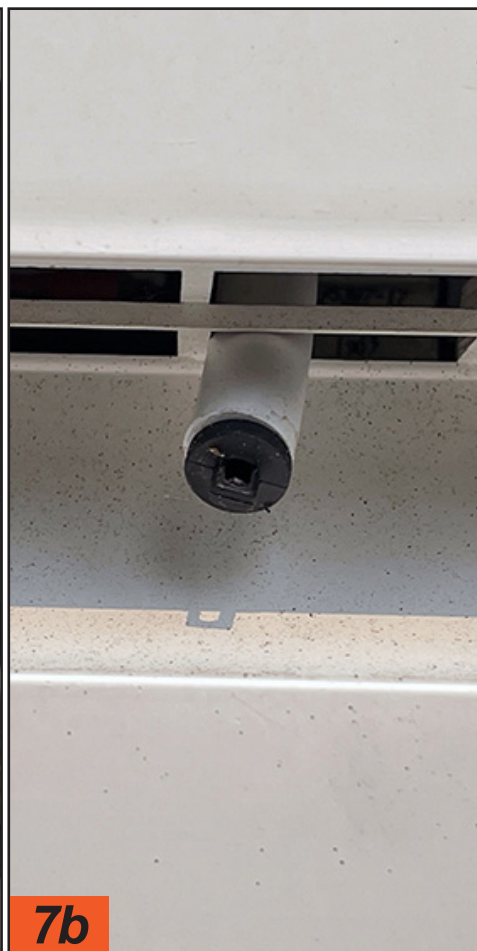
In order to drain condensation from the evaporator/cooling fins inside the refrigerator, a plastic tube is routed from the drain pan below the evaporator to a can mounted in the back of the cooling unit. The heat in this area is designed to evaporate the moisture, but it's best to run this tube out the bottom vent as shown here. This will require that the tube be extended with parts available from any hardware store.
