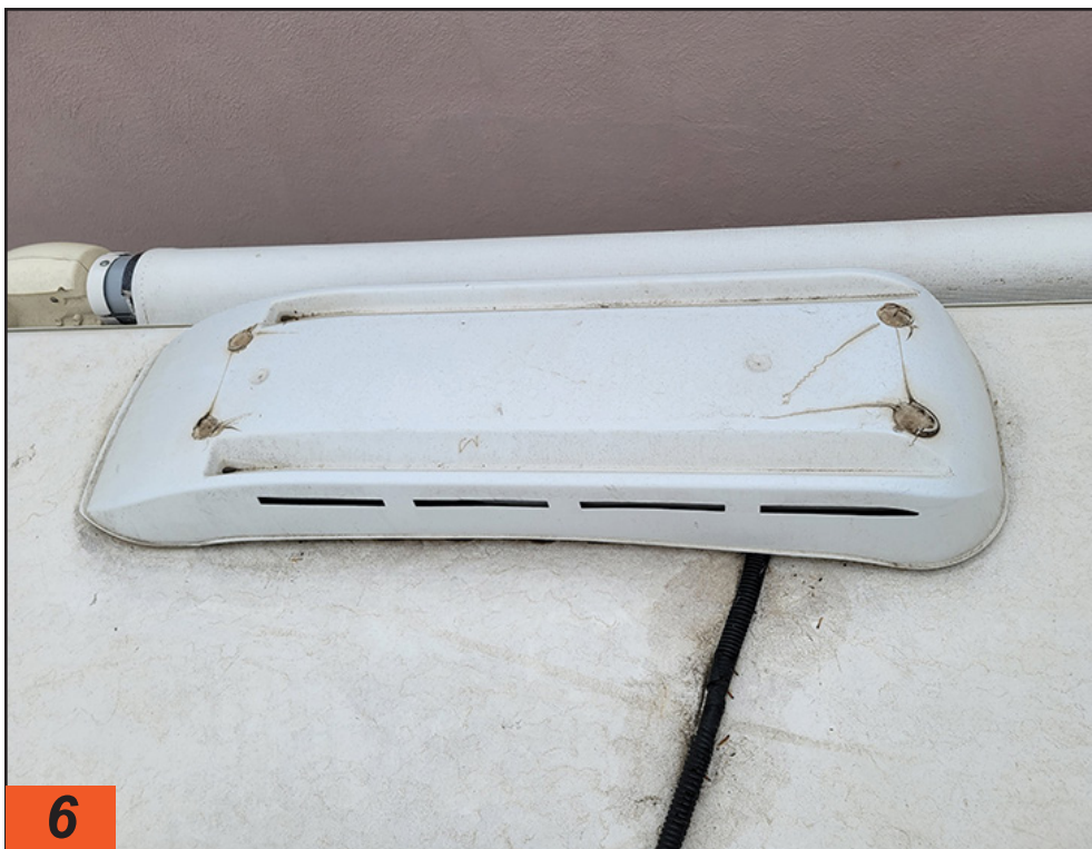
All absorption refrigerators require two vents to evacuate the heat. Refrigerators mounted in a slideout will have an upper and lower vent mounted in the sidewall. Those installed in a solid wall will have an upper vent, like this one, mounted in the roof.
