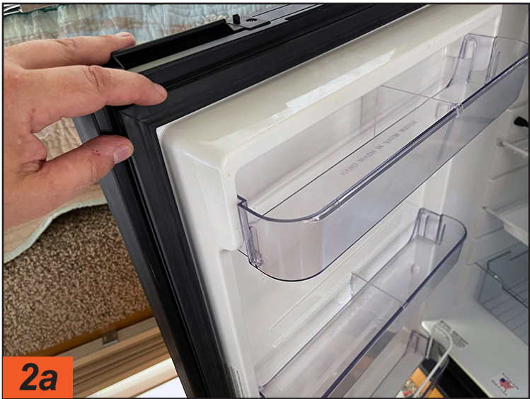
2a 2b The magnetic door gaskets (seal) must be tight to prevent the leakage of cold air. Inspect these gaskets frequently, because replacements are typically not available without buying the whole door. Aftermarket seals are usually not that effective. One simple way to determine if the gaskets are holding is to insert a dollar bill between door and refrigerator frame. There should only be a small amount of resistance when pulling the dollar bill out.
