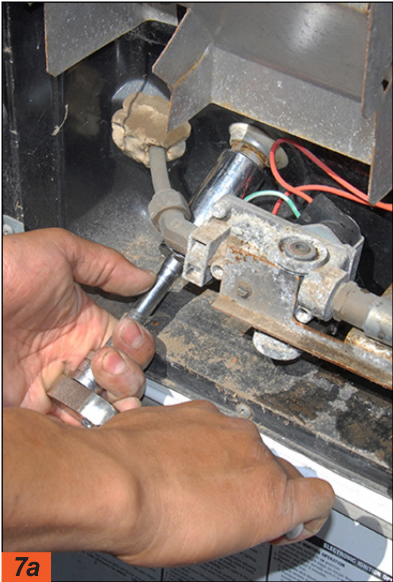
7a The water heater should be drained at the end of every season. Atwood water heaters use a plastic plug that is easily accessed using a ratchet, extension and appropriate socket. This plastic drain plug from an Atwood unit is several years old — note the silt residue caused by water tank corrosion and infrequent maintenance.
