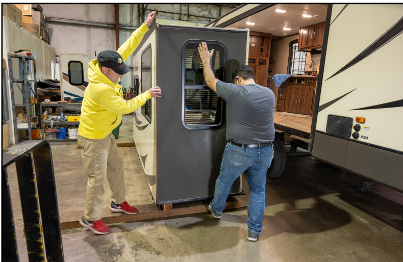
RV slides are both heavy and off-balance, so it's important to have helpers and a forklift to remove them from the coach or trailer.
