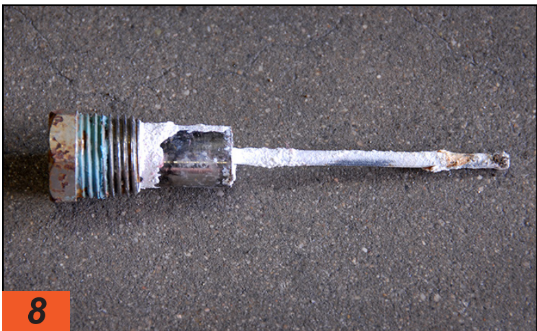
8 All of the magnesium on this anode rod from a Suburban tank has been eaten away by corrosion, leaving only the metal core. Obviously, you shouldn't wait this long to replace the anode rod; it should be checked twice a season for signs of corrosion and replaced when it has lost 50-75% of its material. Be sure to apply anti-seize or Teflon tape when replacing the anode in the water heater.
