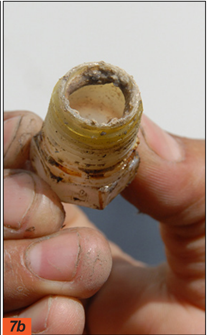
7a The water heater should be drained at the end of every season. Atwood water heaters use a plastic plug that is easily accessed using a ratchet, extension and appropriate socket. This plastic drain plug from an Atwood unit is several years old — note the silt residue caused by water tank corrosion and infrequent maintenance.
