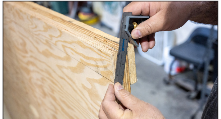
One-inch-thick marine-grade plywood is ideal for use as a replacement sub-floor in RV slides. This type of plywood is highly resistant to water intrusion, and provides a stronger, more rigid floor.
