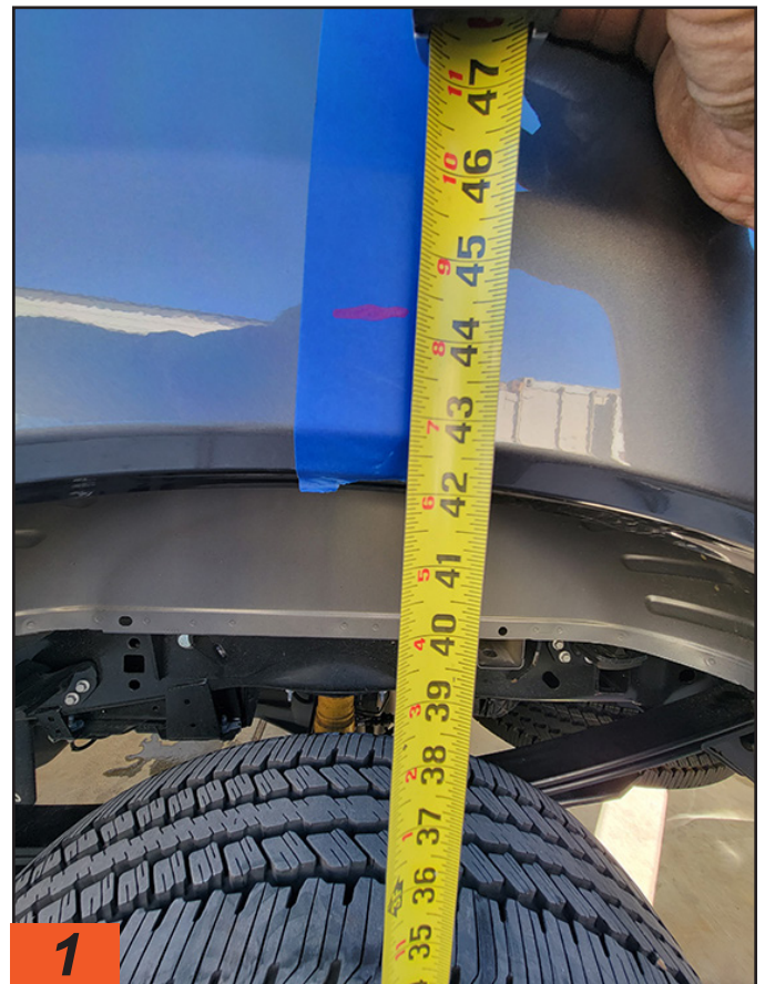
Before installing the hardware, measurements were taken at the rear wheel wells to establish heights from the ground before and after hitching up the fifth wheel — note the painter's tape and marking for repeatability and accuracy. After the installation, the rear end gained 3\frac{3}{4} inches in height with the fifth wheel hitched to the truck.
