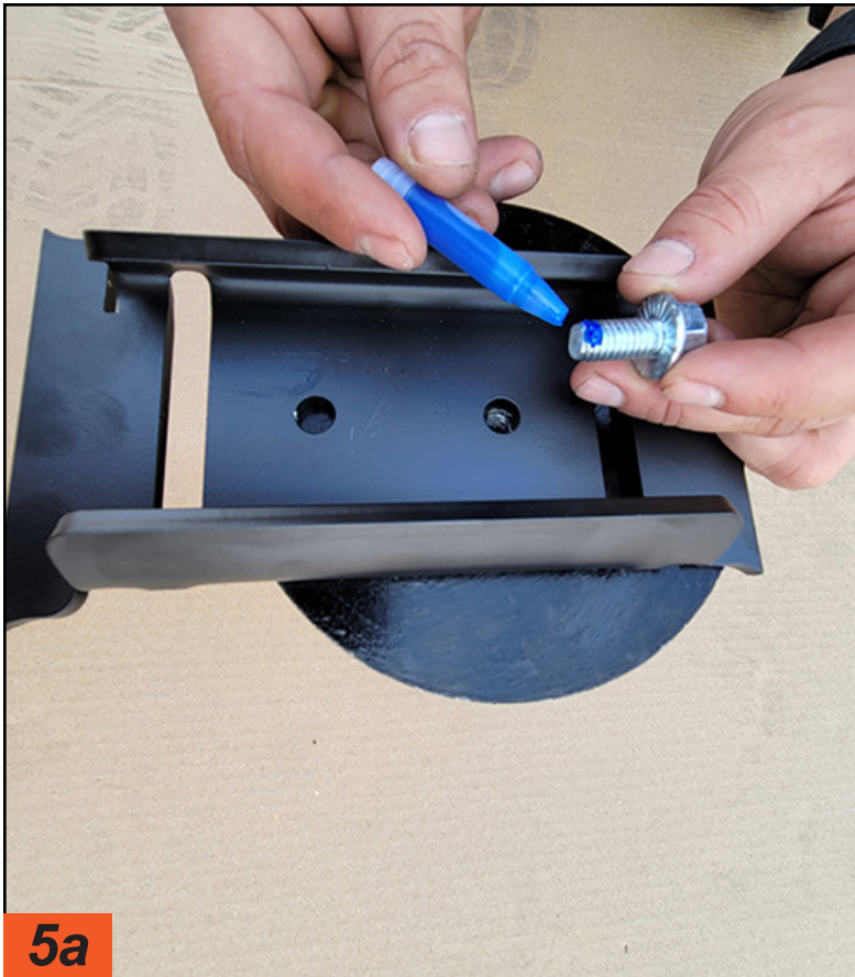
5a Blue Loctite, supplied with kit, was applied to the bolt used to attach the bracket to the bottom of the spring. The bolt was at first snugged just enough to allow the bracket to rotate. This bracket was later U-bolted to the axle housing.
