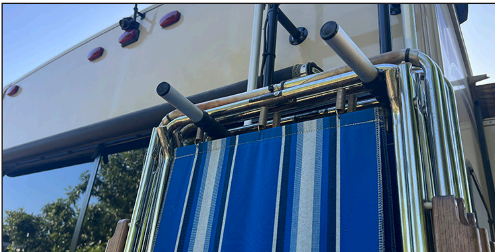
Folding chairs can be placed on the arm extensions in any practical opening between the frame and fabric. The grip on each arm extension provides a quasi-cradle for the chair frame to rest against. After making sure the chairs are tightly packed on the arm extensions, a strap is used to assure they will not move while on the road. RVE
