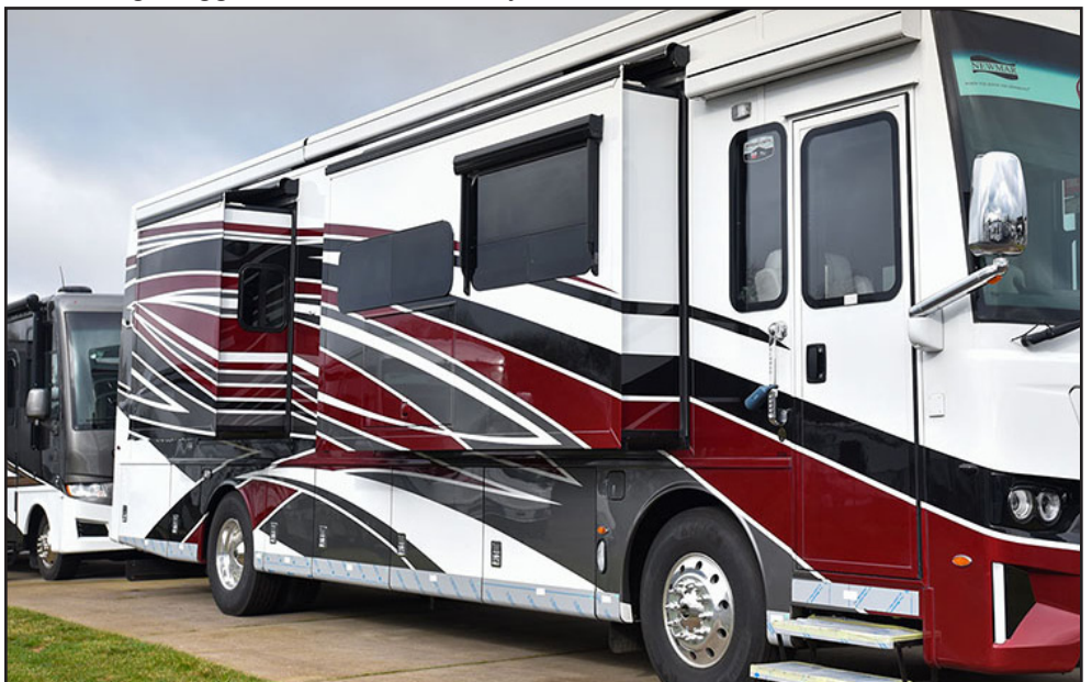
Seals around RV slides are a common source of interior water leaks. The wiper seals have to be kept clean and conditioned in order to lessen the chances of water intrusion from the outside.
