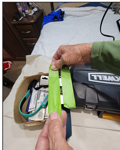
The metal jigsaw foot was covered with painter's tape to prevent scratching the adjacent wood when cutting the hole.
