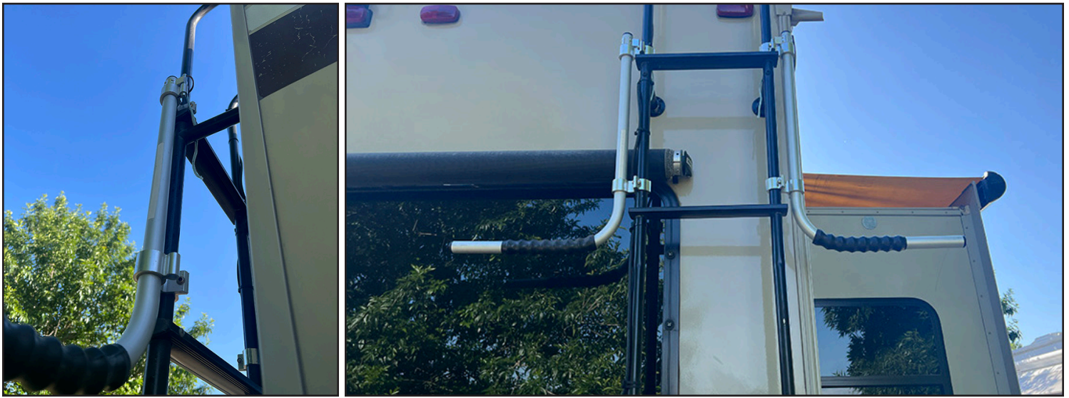
A unique feature is to remove the locking pins from their respective holders, which release the arms and allow them to swing out of the way, freeing the ladder rungs from obstructions.
