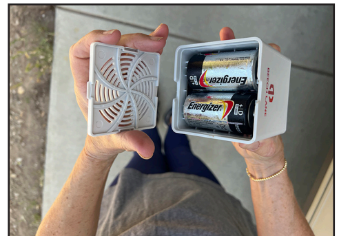
Removing the bottom cover from the housing reveals the battery compartment; two D-cell batteries power the fan motor. According to my friend (who has used the fan for some time now), the batteries last for months; the jury is still out on full-time service. Even so, swapping out batteries once in a while is cheap insurance against possible food spoilage when you're on the road. RVE
