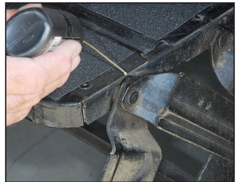
The entry step is one of the most heavily used items on any RV. Inspect for adverse wear and lubricate any moving parts. We like using Tri-Flow Superior Lubricant with PTFE. RVE
