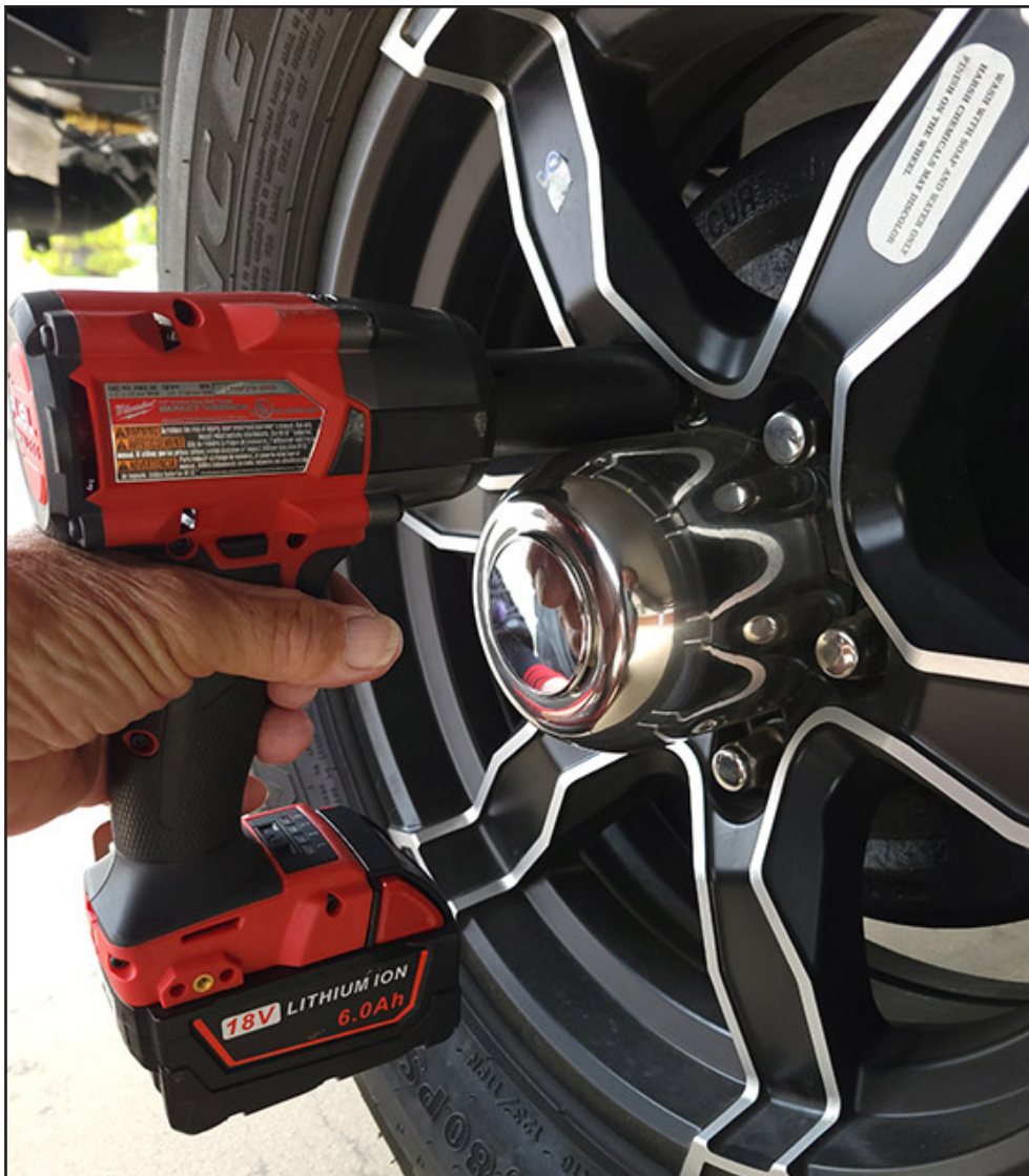
A ½-inch impact gun makes short work out of removing lug nuts, but it's important to get one that has enough torque to meet the specifications for the wheels; usually 100 ft.-lb. is just the starting point for most RVs.
