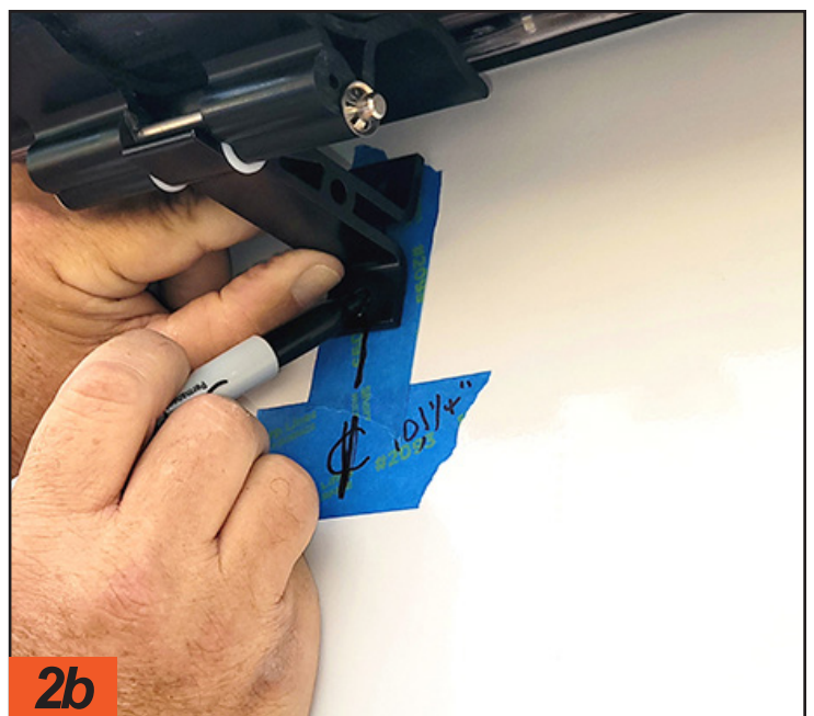
2a Once the center point is established, painter's tape was used to mark the proper location of the cradle assembly. Any marks made directly to the sidewall will likely be permanent. The cradle must be a minimum of 3 inches from the awning rail, with no obstructions. If a light fixture or other obstruction is the center point, the cradle assembly can be moved to either side without impacting performance.
