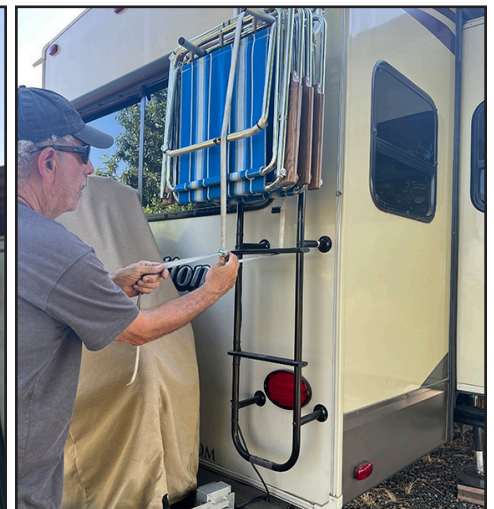
Folding chairs can be placed on the arm extensions in any practical opening between the frame and fabric. The grip on each arm extension provides a quasi-cradle for the chair frame to rest against. After making sure the chairs are tightly packed on the arm extensions, a strap is used to assure they will not move while on the road. RVE
