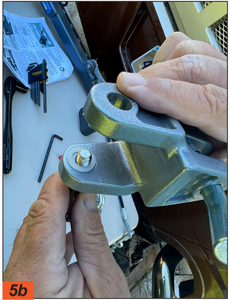
5a Next, one plastic spacer was placed on the new shoulder bolt before maneuvering the swivel ear onto the round nut. The second plastic washer (not shown) was then placed against the other side of the swivel ear as the shoulder bolt was maneuvered into position.
