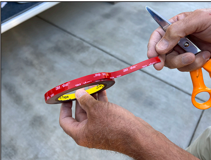
A 33-foot roll of thin 3M VHB acrylic foam tape was purchased at Amazon for $14. This 0.4-inch-wide, double sided tape offers superior holding properties if the surface is cleaned with alcohol beforehand. The VHB tape was attached to the upper and lower flat surfaces on the back side of the molding, in the same manner as the original foam tape. Take your time to make sure the lines are straight and not overlapping the molding edges.
