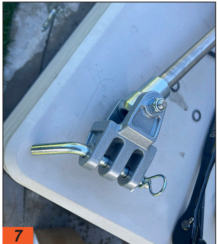
7 Before final tightening of the shoulder bolt, the new swivel ears were checked for proper rotation. If the installation is right, the swivel ear will not rotate more than 10 to 15 degrees in either direction.
