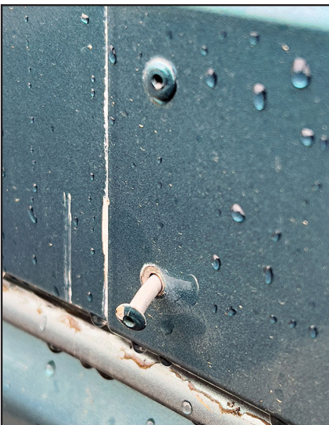
Vibration and flexing of an RV's body often causes seams to come apart, screws to back out and rivets to pop loose. Each is a pathway for water to get inside the walls, ceiling and flooring. Slideout corner cracks are a sign of long-term body flexing, and yet another entry point for water.
