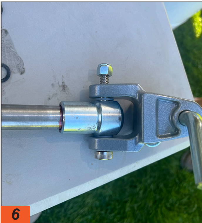
6 The position of the round nut was again confirmed against the earlier marking and the shoulder bolt was ready for tightening. It takes a little finesse to line up the shoulder bolt through the swivel ear, round nut and tow bar arm, so take your time and get it right.
