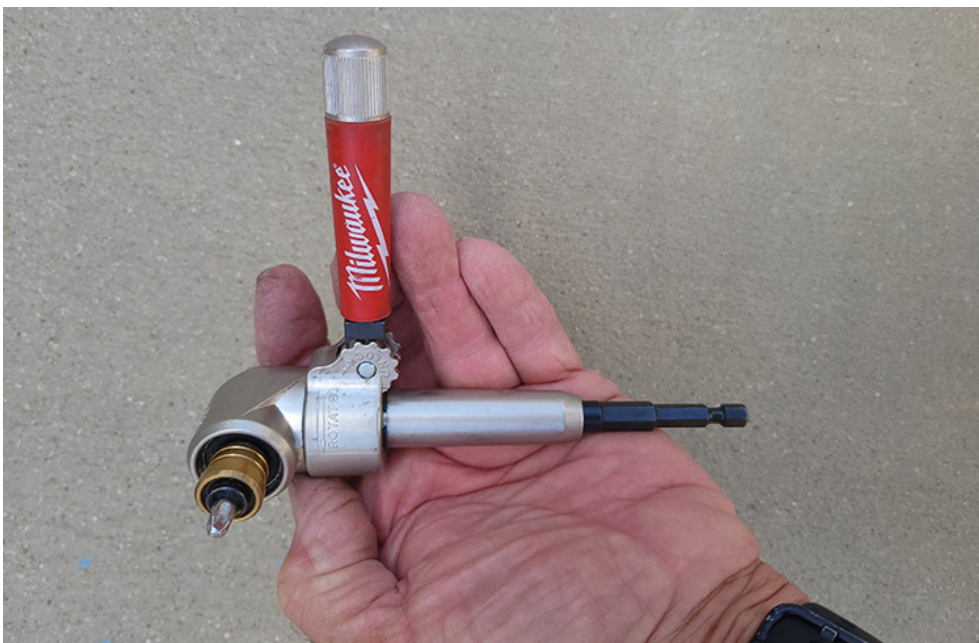
RVs are all about tight quarters and sometimes trying to drive a screw or drill a hole can be challenging without an angle head drill motor. Instead, an angle head attachment can be added to an existing drill, like this one from Milwaukee.
