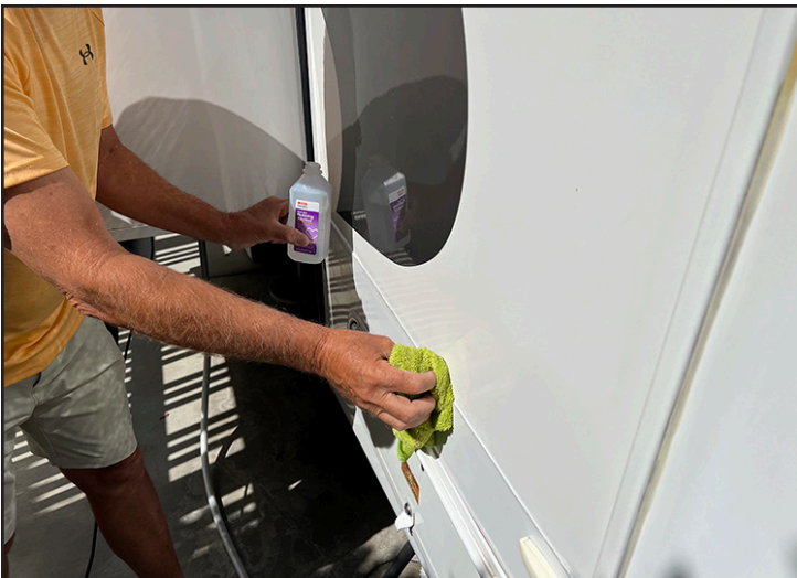
After cleaning the entire length of the sidewall surface with alcohol, the molding was “stuck” to the wall, being very careful to keep the line straight. Finish by running a narrow bead of white silicone along the top and bottom edges of the molding. RVE
