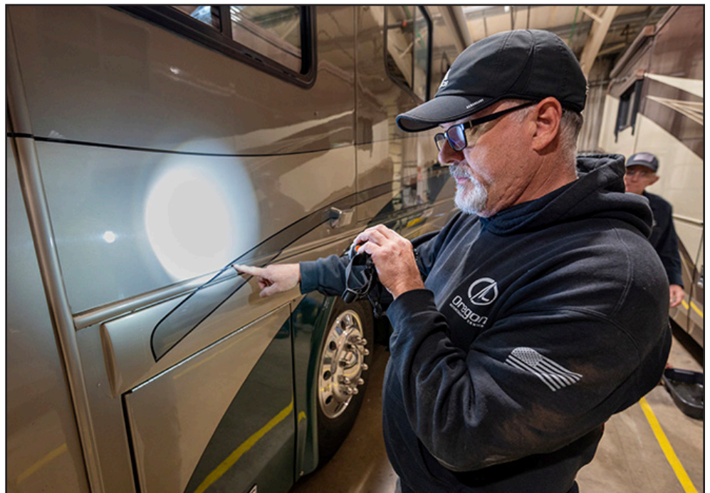
Matt Bryan, Oregon Motorcoach Center's assistant service manager, doing an inspection of a motorhome's exterior and checking for potential water intrusion points along the body molding.
