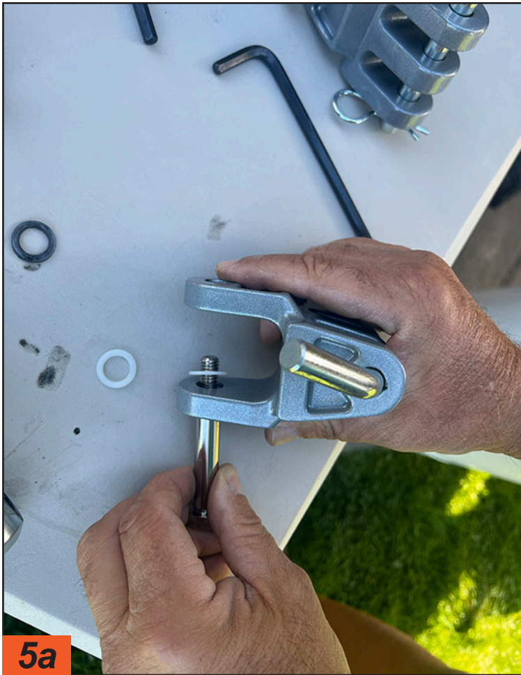
5a Next, one plastic spacer was placed on the new shoulder bolt before maneuvering the swivel ear onto the round nut. The second plastic washer (not shown) was then placed against the other side of the swivel ear as the shoulder bolt was maneuvered into position.
