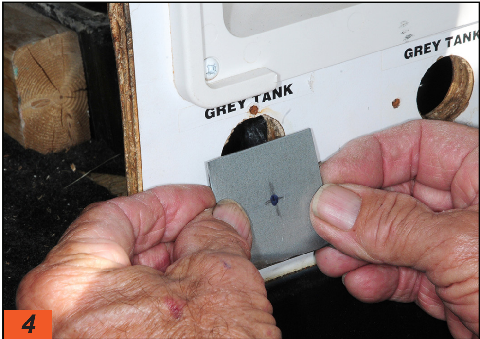
The backing was removed from the two-face tape and the plates were "stuck" to the wall, covering the holes. VHB tape is really strong stuff and the plates will stick forever.
