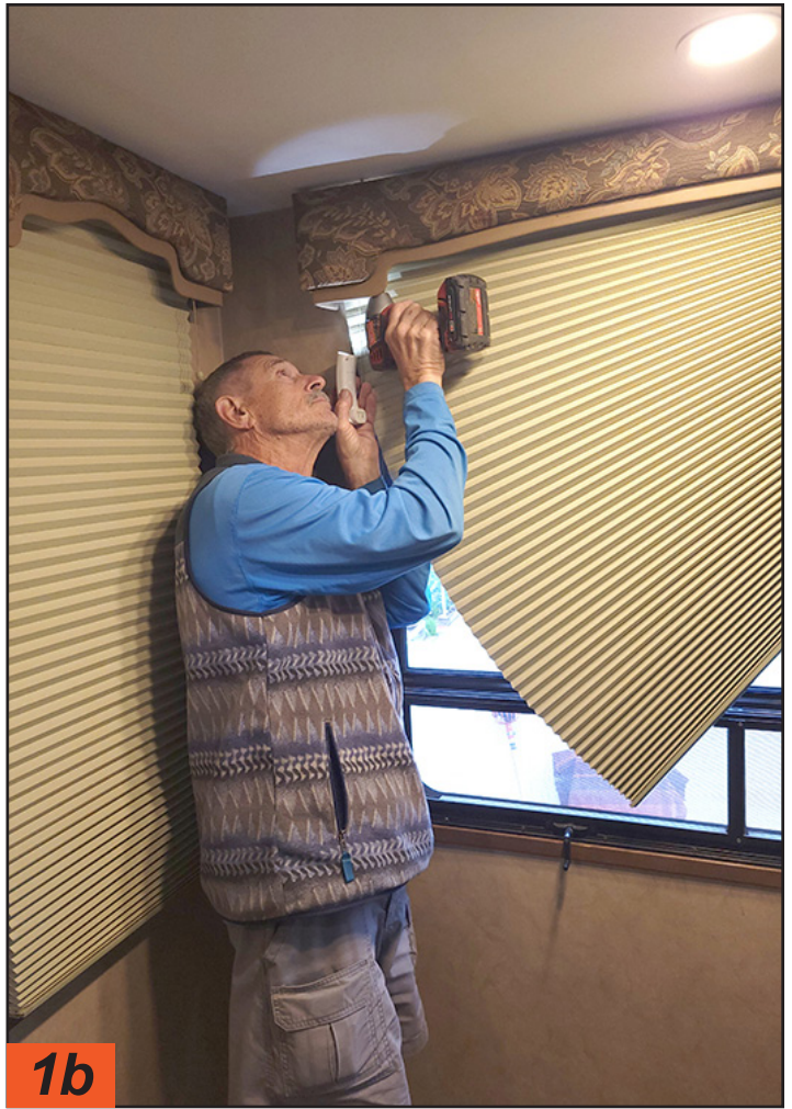
The first step is to remove the valance, which will be slightly different depending on RV model, but most are held in place by a few screws. It's best to use a screw gun or impact driver (on low torque) and a long extension to prevent damaging the valance.
