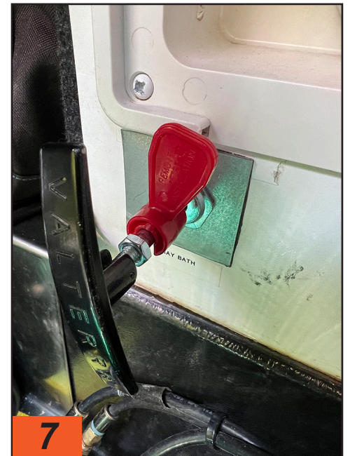
The red tab must be in place when the cable assembly is installed in order to make sure the length is right when cutting the casing and internal wire for attaching to the valve. The cable assembly is secured with a locknut behind the wall and the T-handles can be adjusted for comfort.
