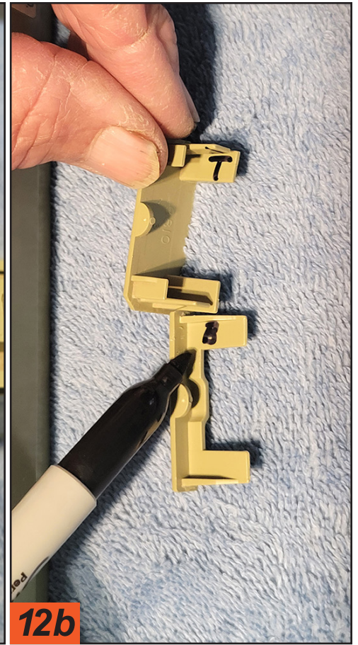
The end stops were removed from the head and bottom rails. It's best to identify the top and bottom end stops with a marker to help with the re-installation. Make any marks in inconspicuous spots.
