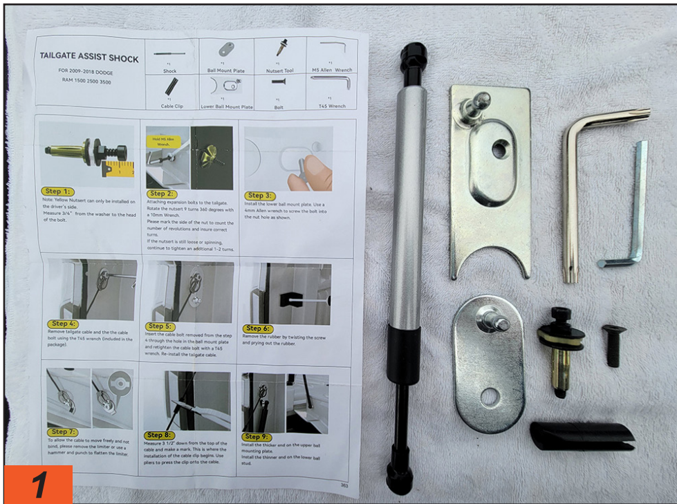
The Tailgate assist kit includes all the parts necessary — and even a couple of rudimentary tools — to install the parts in about an hour. Instructions come with photos but still required some intuition.
