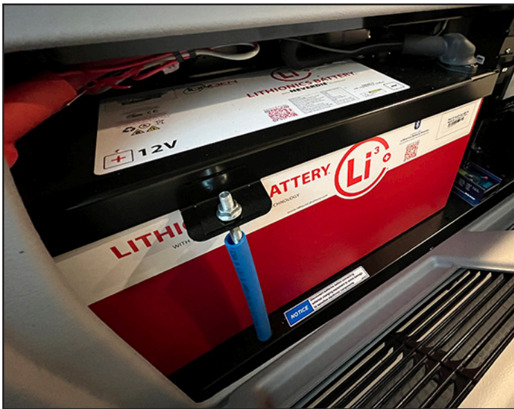
Lithium-ion batteries require special charging algorithms, which the newest inverter/chargers have built into their circuitry.
