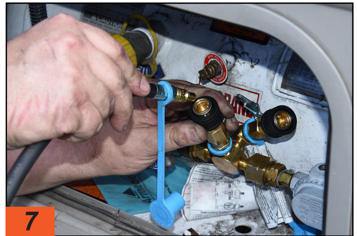
7 When it's time to use an exterior appliance like a gas grill, the collar on the fitting is pulled back and the hose inserted.
