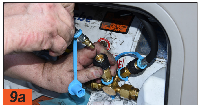
7 When it's time to use an exterior appliance like a gas grill, the collar on the fitting is pulled back and the hose inserted.
