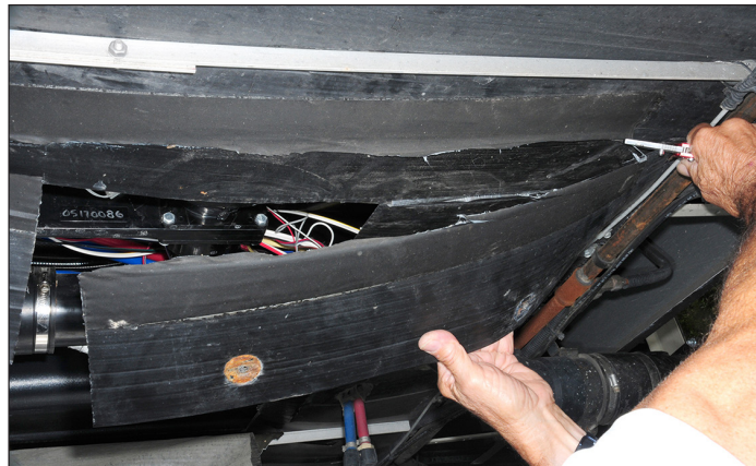
Making the dump valves accessible without having to cut the underbelly will reduce repair time and costs.
