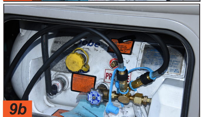
9b If needed, the second line can be attached to supply gas to fuel another appliance.
