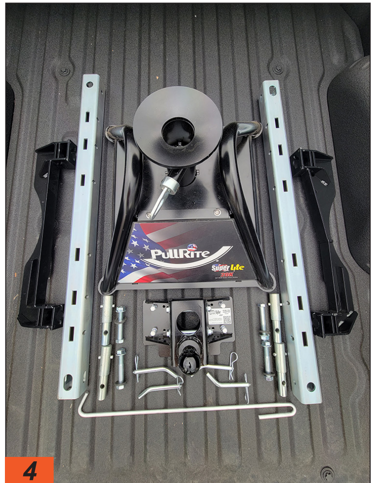
4 PullRite's SuperRail Clean Bed Technology mounting system was ordered with the SuperLite model hitch for the 2023 Ford F-250. The rails bolt into existing holes in the frame and can be removed between trips to free up the truck bed for hauling. One person can usually lift out the 50-pound SuperLite, which is strong enough to tow fifth wheels up to 20,000 pounds.
