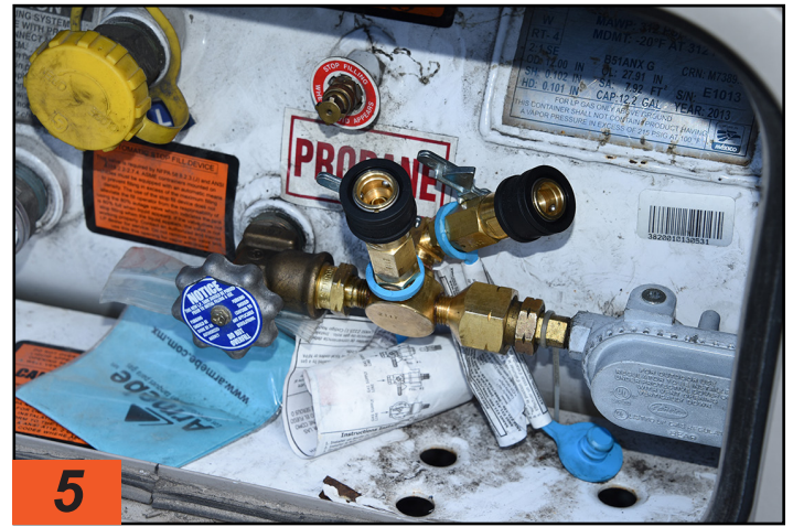
5 Here, the fittings are in place. It may be necessary to rotate them upwards slightly (as shown) so they clear the door when it is closed.
