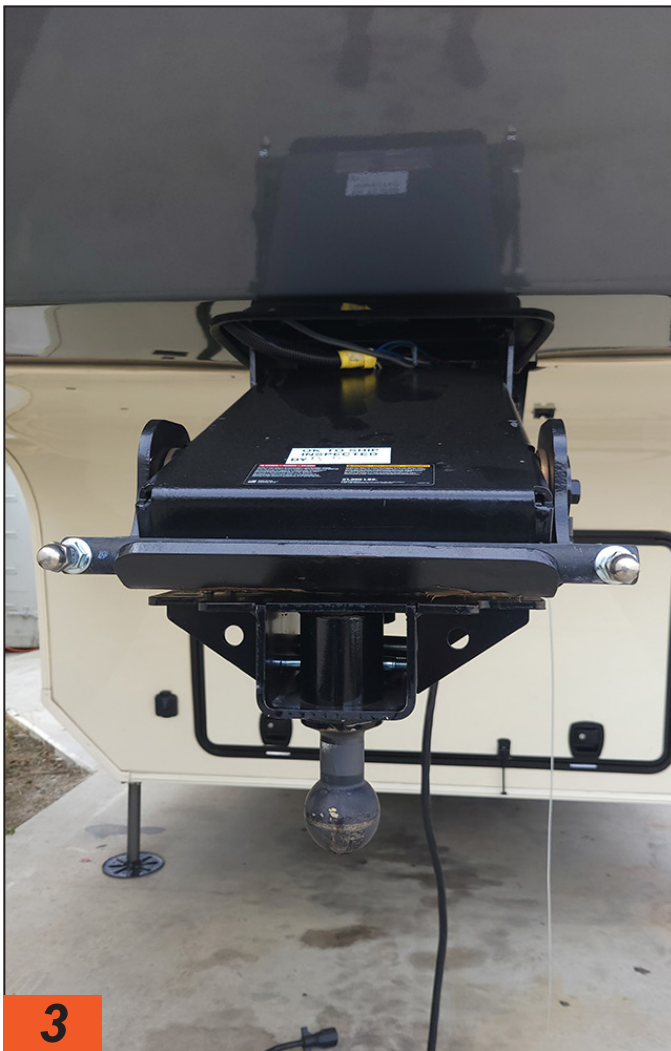
3 A special adapter, part #4446, must be ordered with the hitch for fifth wheels fitted with a Rota-Flex pin box. Installing this bracket will isolate the movement of the pin box, which is necessary when using the SuperLite hitch.
