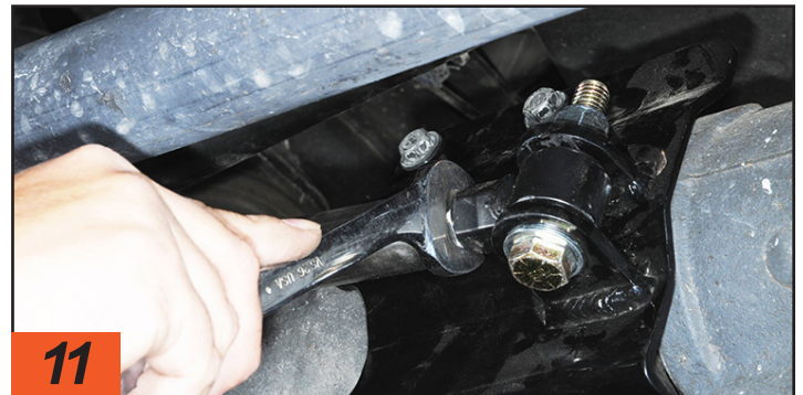
11 Once the jam nuts were tightened against the ring nuts, the truck was test driven to make sure the unit was centered properly. The truck pulled slightly to the left, so the driver's side jam nut was loosened, and the cylinder rotated upward slightly before retightening the jam nut. RVE
