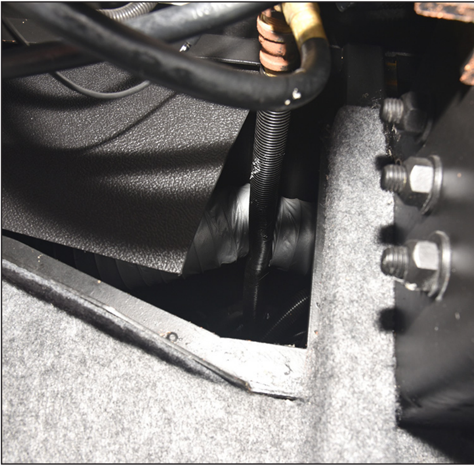
Gaps like this in the storage area of a RV make it very easy for bugs and even larger rodents to pass freely from bay to bay and eventually into the living quarters. Find these and block them with wire screen to restrict their access to your RV.
