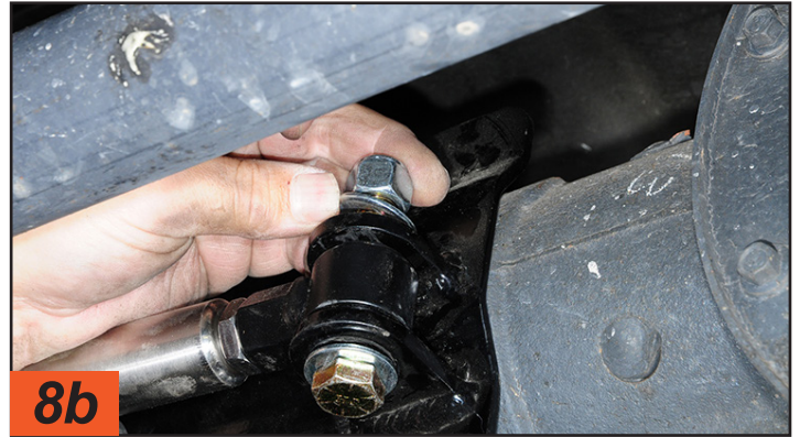
8a It took a little coaxing with a block of wood to get the end of the Exact Center into the axle bracket. There's no question the fit is precise. The stabilizer was mounted into the axle bracket first. A new bolt (provided with the kit) was used here and torqued to 57 ft.-lb. after coating with thread sealer.
