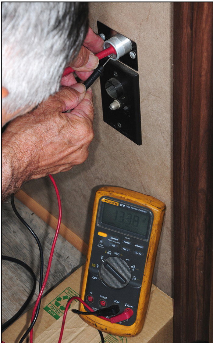
A multimeter is one of the most versatile tools for diagnosing electrical problems. Any 12-volt DC outlet can be checked using the probes correctly. Make sure the probe touching the center contact does not accidentally touch the ground side of the socket or the fuse will blow.
