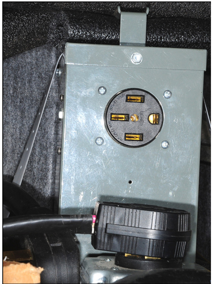
The Hughes Autoformer boosts low voltage conditions at the pedestal. In some cases, it can make the difference on whether or not you can run the air-conditioner in parks with unstable power. This model has been installed in a storage compartment, but the company also offers portable versions, along with high-quality surge protectors.
