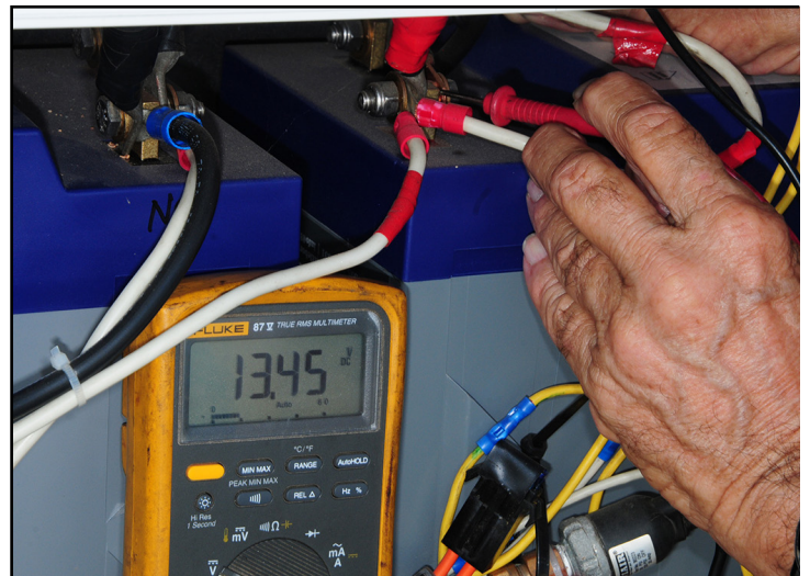
If you suspect a problem with the batteries, the multimeter can be used to probe the terminals for proper voltage. This is where the testing normally begins when low voltage impacts appliance/accessory performance.
