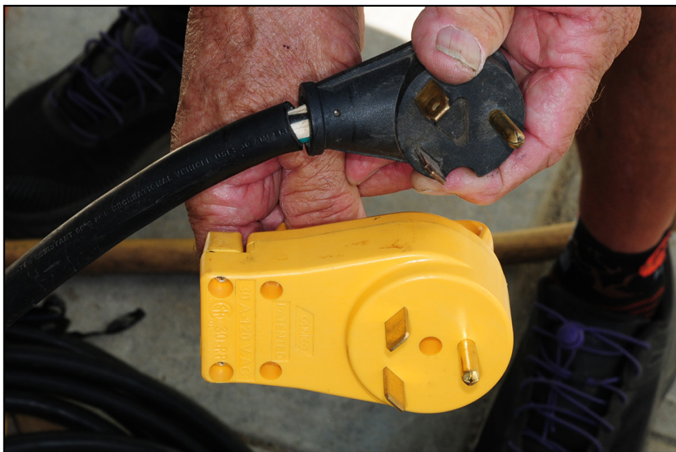
Over time the molded ends of the power cord can pull apart and fail due to water intrusion or wire separation. Replacement ends are available online and at some RV supply stores and can be easily installed.
