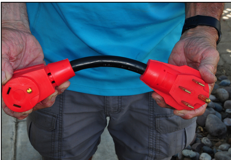
A 50- to 30-amp adapter is one of the most commonly used pigtails among RVers who have 50-amp service. There are many situations when only 30-amp service is provided.
