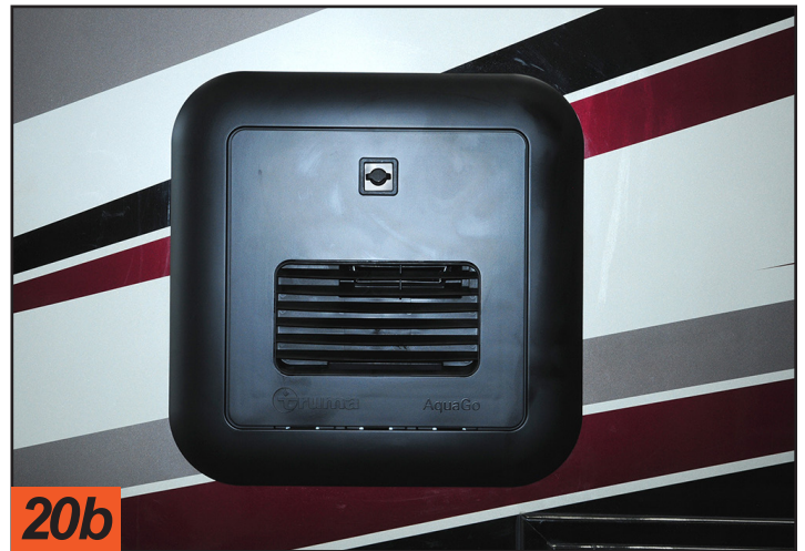
20a 20b The last installation step was to install the access door, which not only looks nice but is also designed to flow fresh air to the burner and exhaust any gas in an efficient manner via an integrated ventilation grid.
