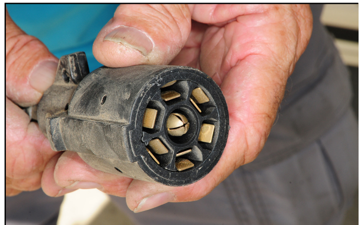
The 7-way Bargman plug from the trailer or dinghy vehicle should be checked for corrosion build-up on the terminals. Start here if the lights and brakes fail to operate properly. Terminals can be cleaned with a brass brush and should be treated with dielectric grease or product that improves continuity, like DeoxIT D100L. RVE
