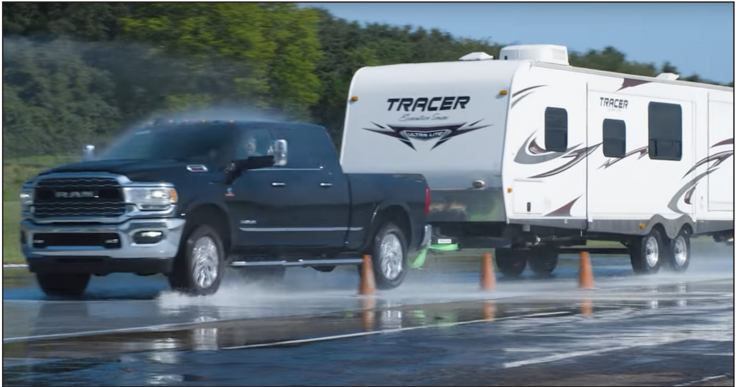
The Lippert ABS was tested extensively at the Navistar Proving Grounds under various conditions.
