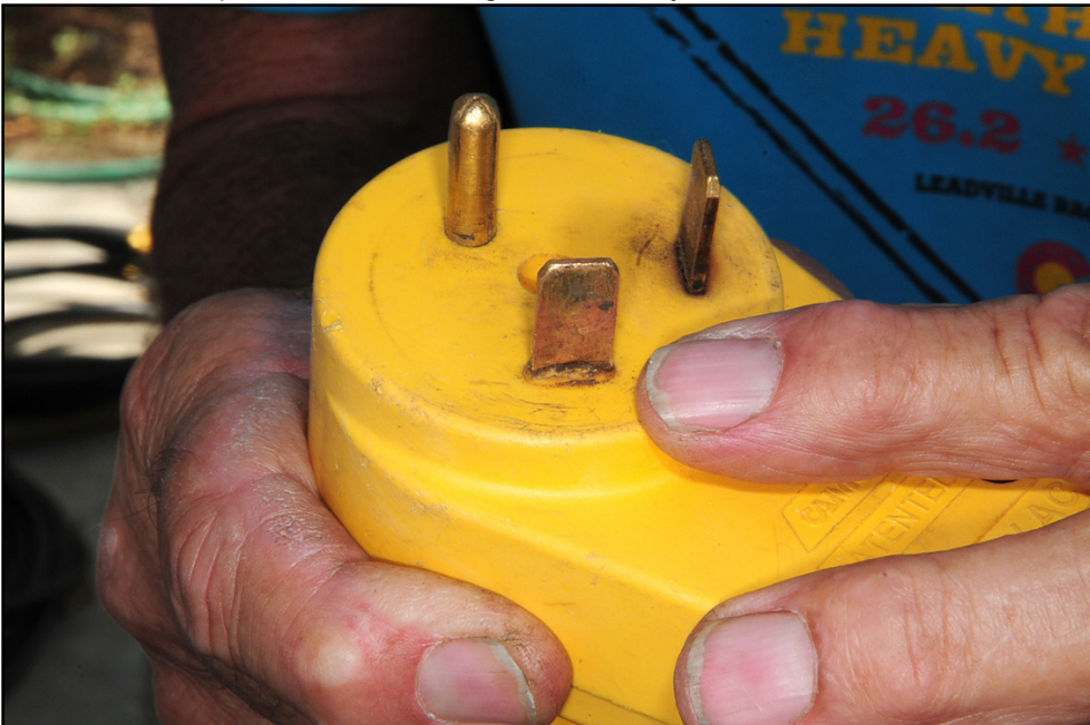
All RVers should carry several power adapters to allow electrical hookup when the pedestal is not equipped with the standard 50- and 30-amp outlets. When these adapters overheat, the prongs can become compromised and will need to be replaced. Always use adapters with pigtails.
