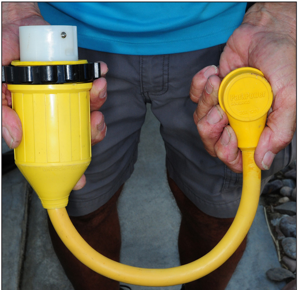
Marinco, a supplier of electrical components to the marine industry, offers high-quality adapters that last a long time under harsh conditions. Shown is a 50-amp plug that goes into the RV's receptacle and has a 30-amp female connector on the other end. Employing this adapter makes it possible to use a 30-amp power cord rather than lugging the 50-amp version when only 30-amp service is available.
