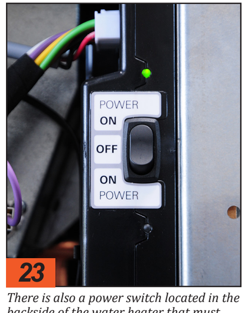
23 There is also a power switch located in the backside of the water heater that must be turned on to operate the water heater. This switch is left on so the water heater can be controlled at the remote panel. A green light here will flash a code if there is a malfunction. RVE
