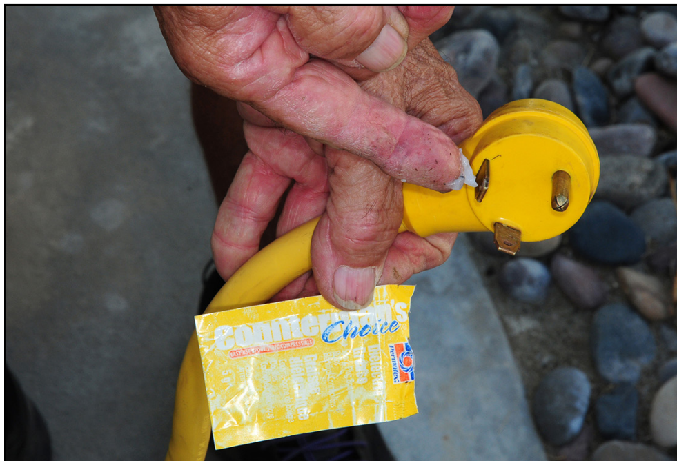
Adapter ends can be difficult to pull apart from the power cord or pedestal outlet. Coating the prongs with dielectric grease not only protects against corrosion but makes it easier to plug and unplug.
