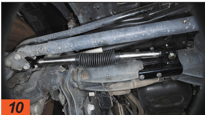
10 The Exact Center stabilizer can be installed in either direction and is designed to resist steering wander by keeping the system pressurized.
