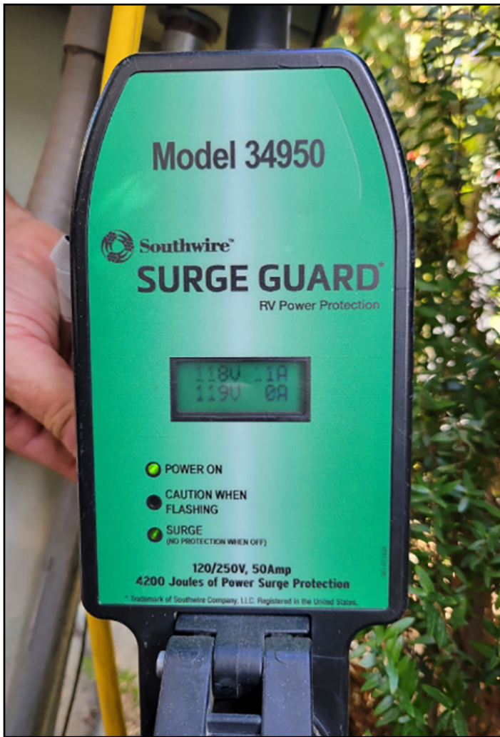
Many portable surge protectors provide information on power conditions at the hookup pedestal. This device from Surge Guard monitors power condition while protecting against voltage variations from lightning and brownouts.
