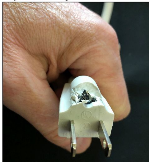
Never cut off the ground pin of an extension cord, and never use a cord with a missing ground pin.
