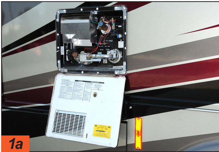
1a The original hot water tank in this motorhome was in good shape, but the owners were full-timers and wanted the convenience of on-demand hot water. The door was removed from the original water heater to begin the process releasing the housing from the side-wall.
