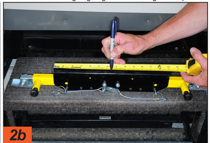
Center points for the bottom step and the SolidStance frame were measured and marked to make sure the hardware could be oriented properly.
