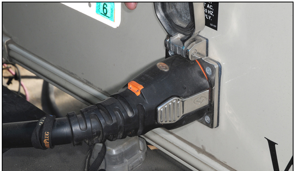
Looking for a better connection? The Smart Plug power cord system ( www.technorv.com ) is one of the best in the business. It uses a completely different plug and receptacle and improves continuity without arcing. Kits to replace the ends of your existing power cord are available in 50- and 30-amp versions.
