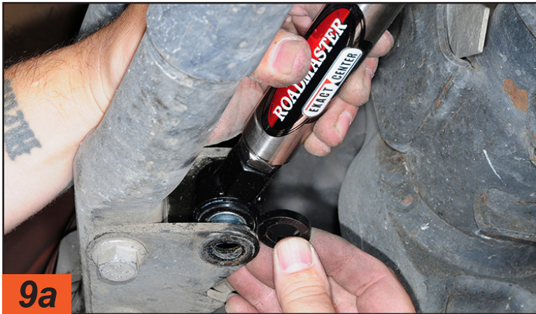
9a Since the factory tie-rod bracket is a little wider than the Roadmaster replacement, a washer/spacer is provided with the kit to take up the slack. The original bolt, washers and nut are reinstalled in the tie-rod bracket to hold the end of the Exact Center stabilizer in place. This nut and bolt are also torqued to 57 ft.-lb.
