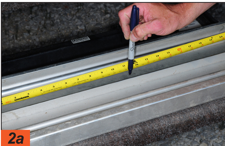
Center points for the bottom step and the SolidStance frame were measured and marked to make sure the hardware could be oriented properly.
