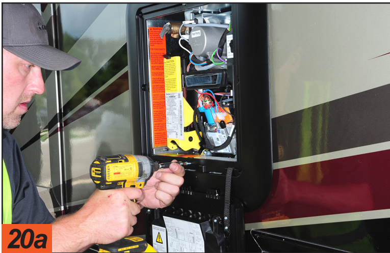
20a 20b The last installation step was to install the access door, which not only looks nice but is also designed to flow fresh air to the burner and exhaust any gas in an efficient manner via an integrated ventilation grid.
