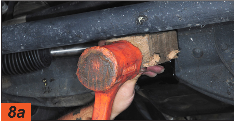
8a It took a little coaxing with a block of wood to get the end of the Exact Center into the axle bracket. There's no question the fit is precise. The stabilizer was mounted into the axle bracket first. A new bolt (provided with the kit) was used here and torqued to 57 ft.-lb. after coating with thread sealer.
