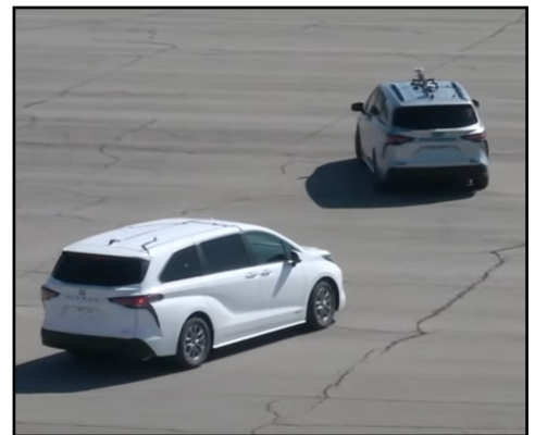
Two vehicles explore the feasibility of "hitchless towing." While both of these vehicles have drivers in them for safety during evaluation, everything is being controlled by the lead vehicle.
