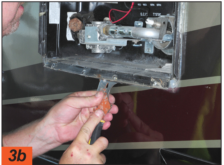
3a The screws were removed from the frame and the old sealant was cut with a scraping tool to release the water heater from the opening in the sidewall.
