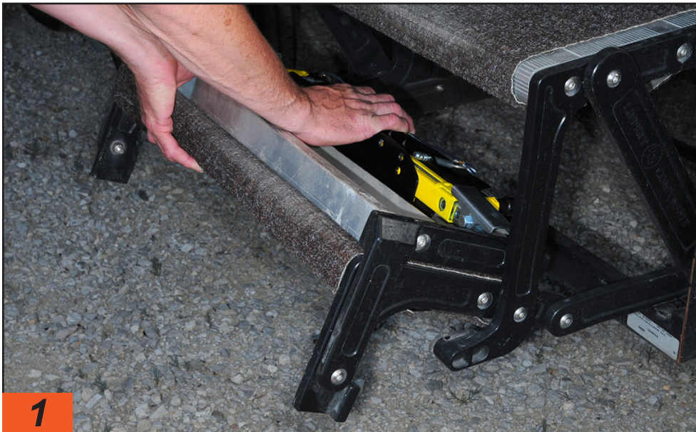
The stabilizer was installed on Lippert's Aluma-Tread triple-steps. It can also work on double step configurations but is not designed for four-step models. Before starting the installation, the SolidStance was held in place and the steps retracted to establish proper clearance.
