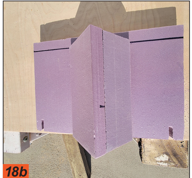
Before taping the wedge assembly, check to make sure it is centered on the bottom and will fit correctly without making additional cuts. Side and top views are shown.
