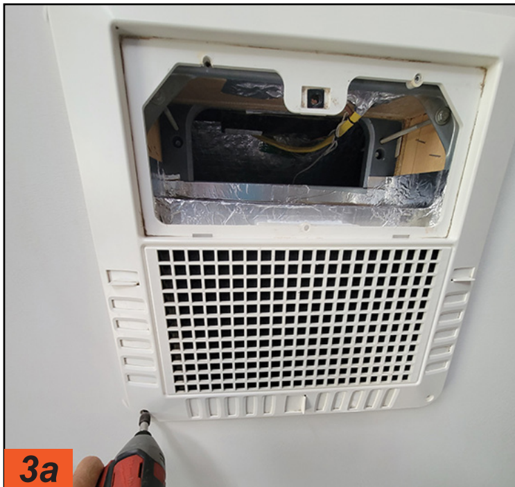
The ceiling assembly is pulled to get better access for cleaning the evaporator. Normally, there are four to six screws holding it in place. It can be on the heavy side, depending on the model. This model has a steel plate, which adds to the weight. You don't want to drop and damage this ceiling assembly because the replacement cost is expensive.
