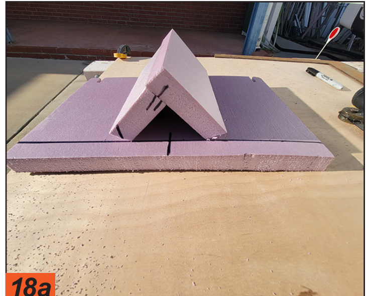
16 Before taping the wedges into place permanently, make sure the bottom plate fits properly in relation to the two upper wedges.
