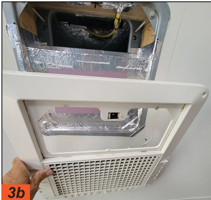
The ceiling assembly is pulled to get better access for cleaning the evaporator. Normally, there are four to six screws holding it in place. It can be on the heavy side, depending on the model. This model has a steel plate, which adds to the weight. You don't want to drop and damage this ceiling assembly because the replacement cost is expensive.
