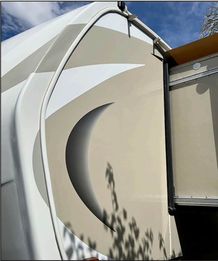
Oxidation was evident after cleaning, following the pattern of the sidewall frame. Here, the oxidation was caused by constant exposure to strong sun and was only a problem on one side. Otherwise, the fiberglass held up fairly well over the five years since the fifth wheel was new — and looks near-new again afterward.
