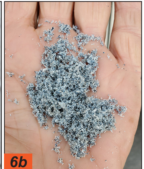
While the 3M wheel is very effective in removing vinyl, it wears down fairly quickly. Most of the time the job requires five to eight wheels. The removal wheel grinds up the vinyl material into tiny pieces, which will make a mess, and the adhesive allows the ground-up vinyl to stick to everything.
