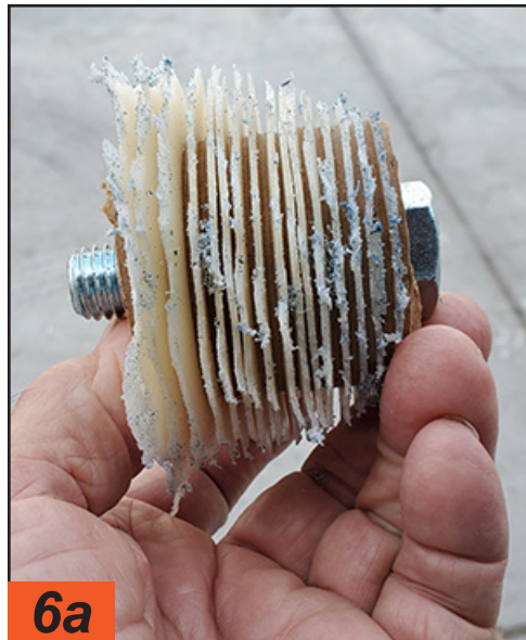
While the 3M wheel is very effective in removing vinyl, it wears down fairly quickly. Most of the time the job requires five to eight wheels. The removal wheel grinds up the vinyl material into tiny pieces, which will make a mess, and the adhesive allows the ground-up vinyl to stick to everything.
