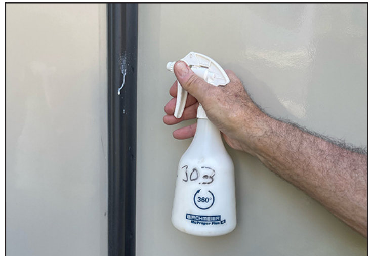
Spraying the slide-out bulb and wiper seals with Aerospace 303 Protectant will protect the rubber over the long run, and make sure moisture and air leaking through the slide-outs are kept at bay. (And no, it doesn't come in this bottle — we bought it in a gallon container and transferred it to this type bottle, which we've found works easier when spraying at different angles.)
