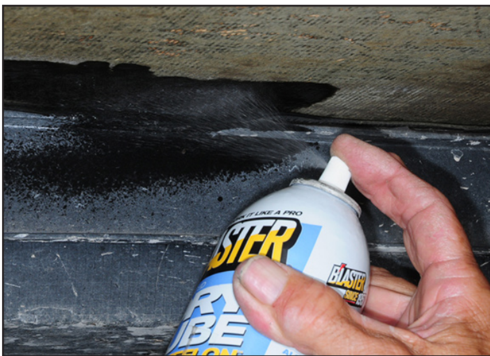
Blaster Dry Lube with Teflon does a great job of lubricating the surfaces at the confluence of the RV and slide-out floors. Normally there's a little more space between the surfaces, but in this case, they were touching and making annoying noises, which were quieted with the dry lube.
