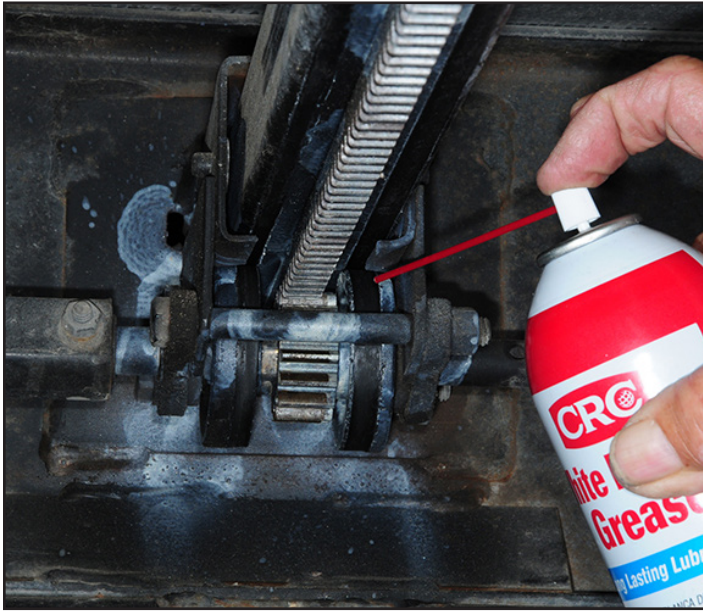
Spray the gear pack liberally, but don't go crazy. Overloading the components with too much lubrication only makes a mess.
