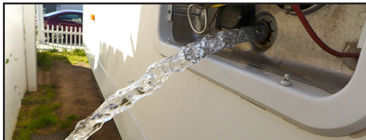
Flushing the hot water tank on a regular basis will prevent build-up of debris, which can alter capacity over time and present a good opportunity to replace the anode rod in Suburban models, if necessary.
