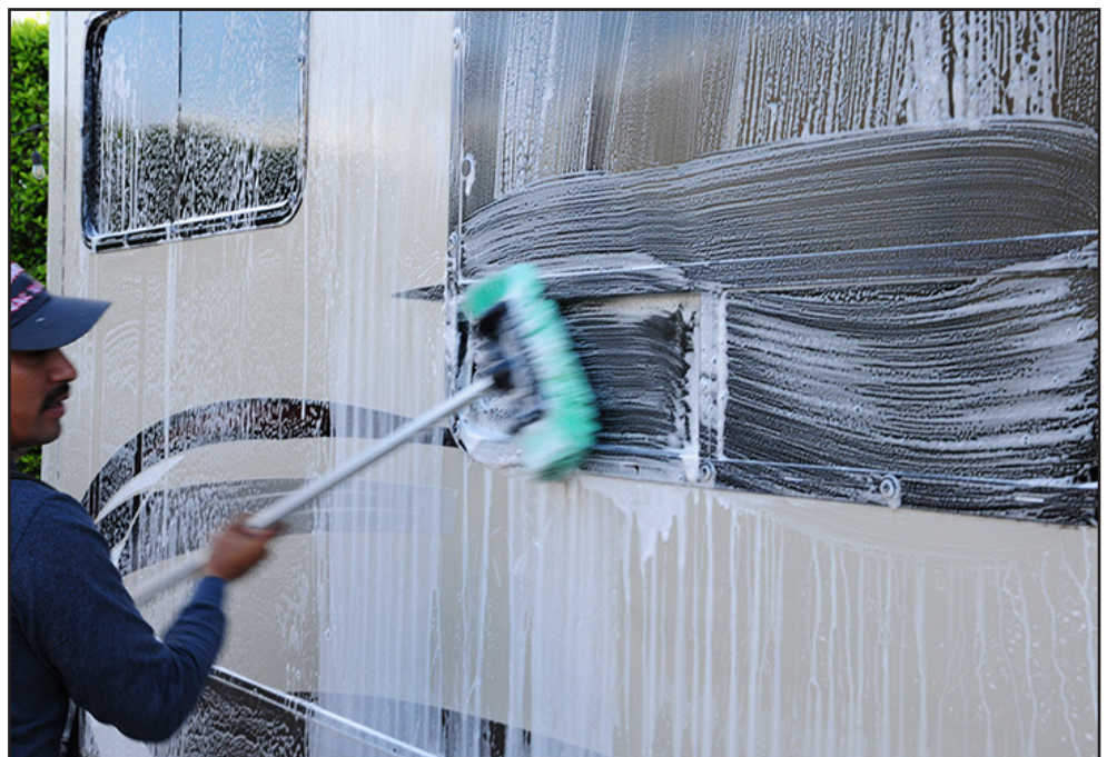
A brush specifically designed for painted surfaces and can be attached to a telescoping handle, which makes it possible to reach the higher sections of the sidewalls and end caps. Once the soap is brushed thoroughly, it must be completely washed off with clean water. This is another area where a pressure washer really comes in handy—and conserves water at the same time.
