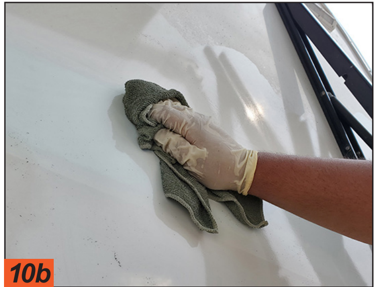
10a When the vinyl and adhesive are dried by the sun and stick to the sidewall, the chemical may not completely remove the residue. When that happens a fine steel wool pad is used to loosen the residue, which is followed with a final wiping with a cloth impregnated with a mixture of alcohol and water.
