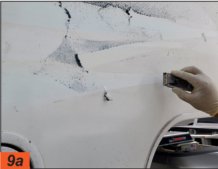
9a Dealing with the residue seems like a never-ending task. It takes a number of passes with the scraper to remove most of the residue, and the adhesive remover is used repeatedly to clean the blade.
