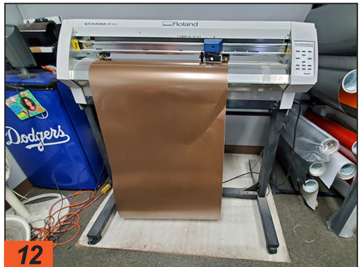
11 V.I.P. Enterprises retains all of the patterns from the original job, which makes it easy to retrieve sections of vinyl. This computer program is always used to duplicate the original graphic design. 12 The replacement vinyl decals are printed from computer-generated graphics the exact pattern is cut for replacement, which eliminates shadowing.
