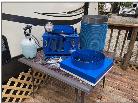
The Sealtech system features a patented fan unit with pressure gauge, plenum and roof vent attachments. The technician will use a sprayer with a mixture of Dawn dishwashing detergent and water to spray around potential incursion points, and document the leaks by taking photos with a smartphone.
