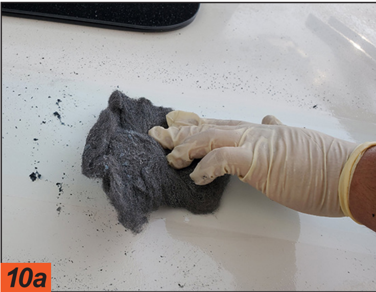
10a When the vinyl and adhesive are dried by the sun and stick to the sidewall, the chemical may not completely remove the residue. When that happens a fine steel wool pad is used to loosen the residue, which is followed with a final wiping with a cloth impregnated with a mixture of alcohol and water.
