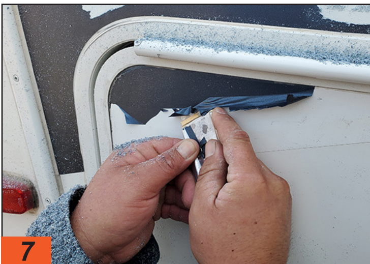
A razorblade scraping tool is used to remove vinyl in tight places, like around the compartment door frame.
