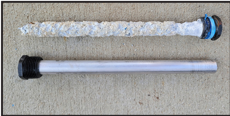
Clearly, the anode rod in this tank was ready for replacement. If the anode rod is ignored, which is easy to do, the steel tank can develop holes and water will leak out, eventually making a mess and possibly encouraging dry rot.
