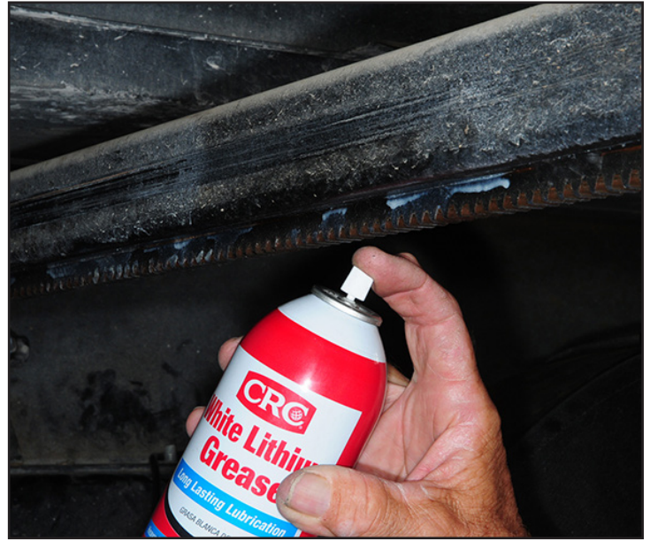
The front and rear racks should be sprayed with the CRC White Lithium Grease along the teeth cut into the steel arms.
