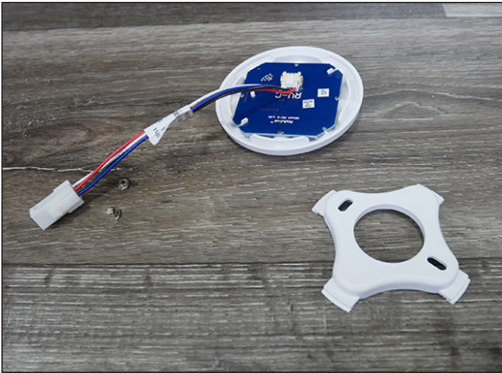
The heart of the JayVoice system is the Modulus Director, developed in conjunction with BMPRO and American Technology Components, which ties into the unit's RV-C communications protocol.
