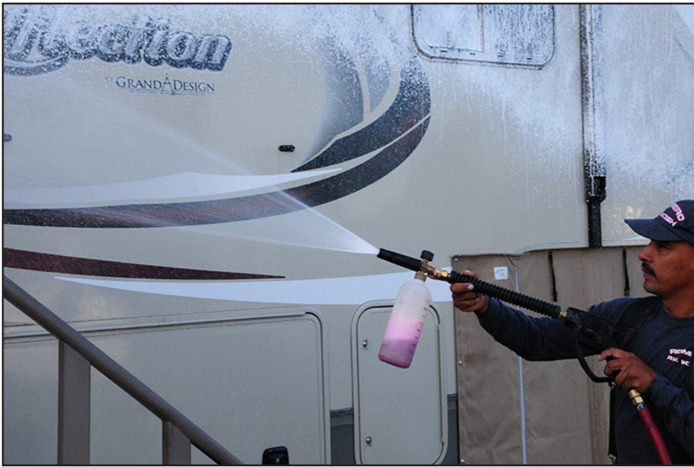
A pressure washer and foaming gun will make it easier to cover larger areas with soap. Foam clings to the surface longer and does a great job of cleaning.
