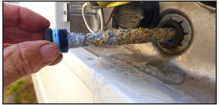
It best to replace the anode rod in a Suburban water heater when the material is 50% consumed. Magnesium rods are best for harder water and not needed in Atwood tanks, which are aluminum. The anode rod is a sacrificial metal to prevent deterioration of the porcelain-coated steel tank used in Suburban water heaters.
