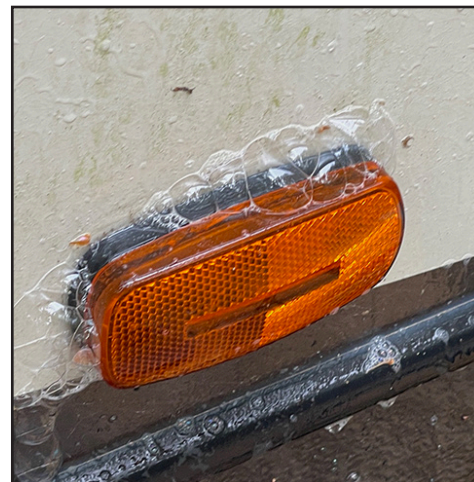
Once sprayed, the bubbles show where air is escaping, indicating a possible leak. Not all bubbles will be a leak in need of repair — and don't be surprised to see bubbles at places you might not expect. This marker light might be a concern and looked at more closely, although the air may be passing inside the fixture from the lamp base and/or wiring run, which may not be a cause for worry.
