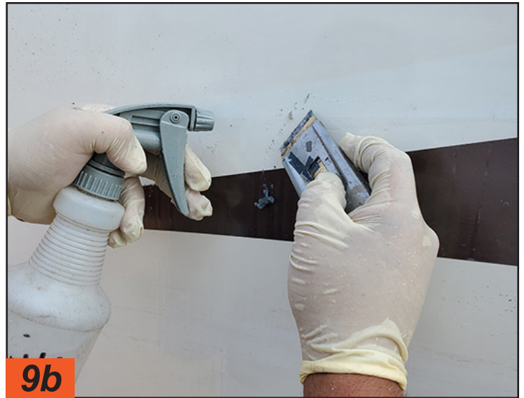
9a Dealing with the residue seems like a never-ending task. It takes a number of passes with the scraper to remove most of the residue, and the adhesive remover is used repeatedly to clean the blade.
