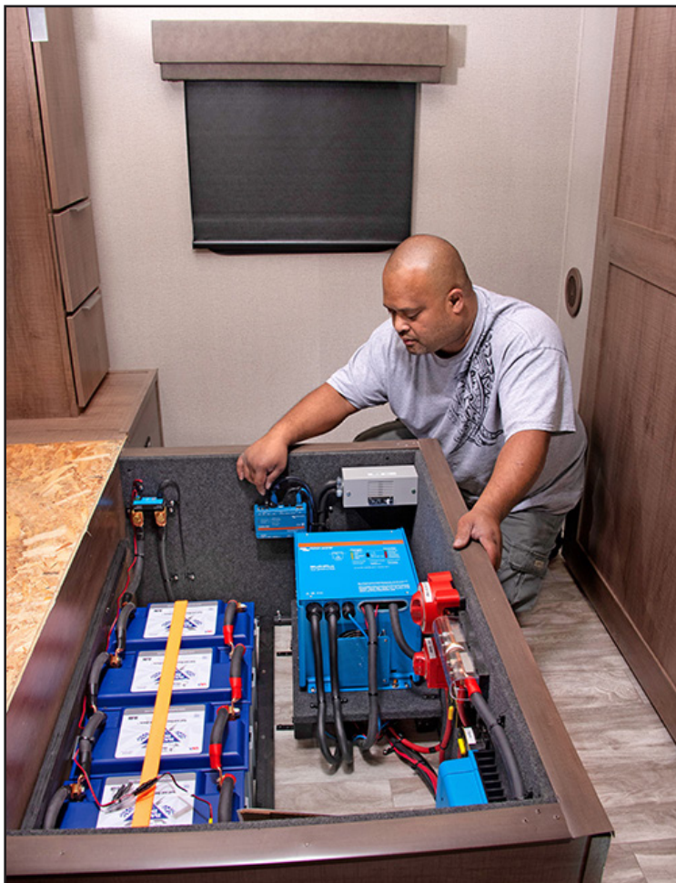
AM Solar master technician Alvin O'Daol checks final connections on an 850-watt solar system installation added to a Grand Design Imagine travel trailer. Photo by Chris Hemer.
