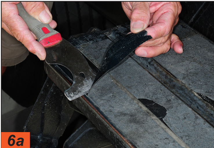
A metal putty knife was used to remove the old grip tape. It takes a while to remove all the tape and if you get lucky, large chunks at a time will pull off the step surface. Once the tape is removed, take the time to wash the steps thoroughly and repaint to restore the finish.
