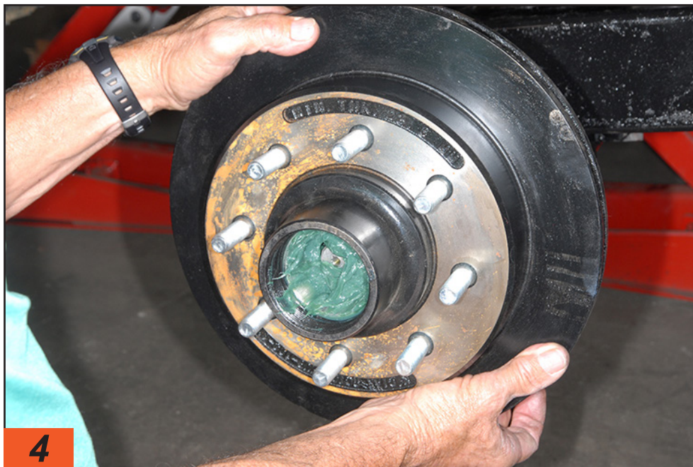
Rotors are positioned on the spindles. Here 13-inch rotors with the Dacromet coating (to minimize corrosion) have 9/16-inch studs, eight on 6 ½-inch bolt pattern, typical of fifth wheel trailers in this size category.
