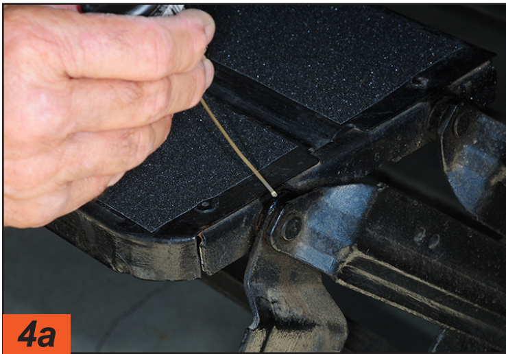
A few drops of Tri-Flow lubricant is applied to the joints in the entry steps. The drip bottle and plastic straw help control the flow of lubricant.
