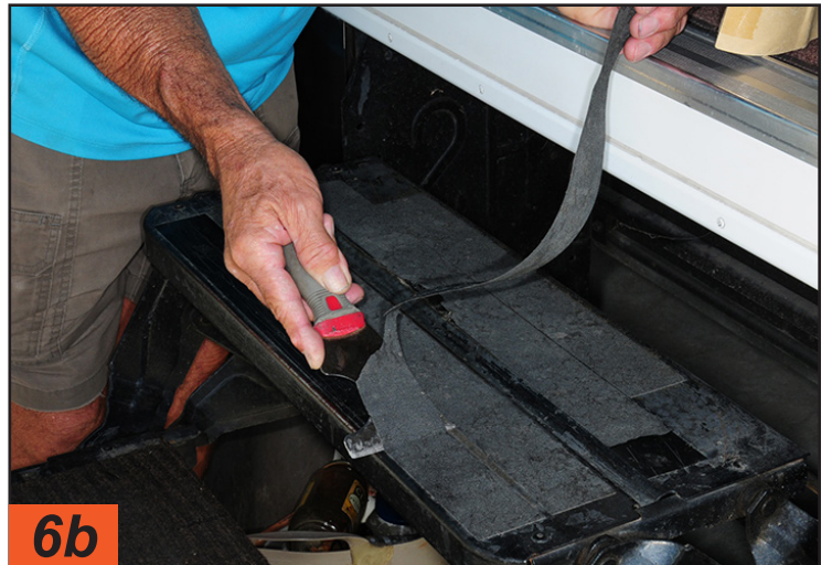
A metal putty knife was used to remove the old grip tape. It takes a while to remove all the tape and if you get lucky, large chunks at a time will pull off the step surface. Once the tape is removed, take the time to wash the steps thoroughly and repaint to restore the finish.
