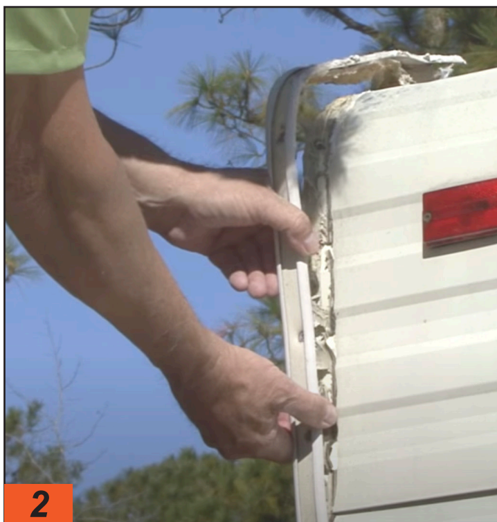
2 With the screws removed, carefully disengage the molding from the corner. Be careful to not bend or kink the molding so it can be reinstalled.
