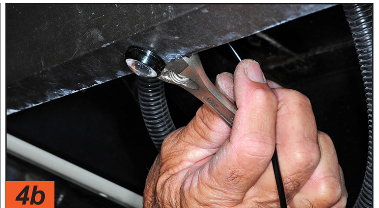
The metal retaining nut is run up the wire to hold the light in place. It can be a little awkward to maneuver the wrench to seat the retaining nut due to the skirt lip angle and surrounding hardware/components. Using a metal nut on aluminum threads could lead to galling, which would make removal difficult. Our worries were short lived, since the thread tolerances are rather sloppy (but still close enough to secure the light without wiggling).
