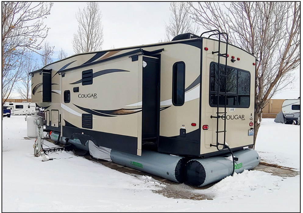
Airskirts are new to the RV world. These inflatable bags come in a variety of sizes and kits specifically designed for different trailers from Airstreams to fifth wheels. Airskirts can be installed under the trailer in less than 15 minutes, according the manufacturer. (Photo courtesy of Airskirts)
