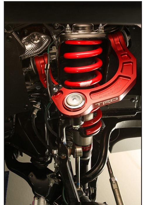
Toyota engineers managed to increase road clearance by two inches compared to a stock Tacoma TRD Sports pickup; the suspension incorporates billet TRD upper control arms.
