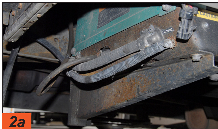
Moving underneath the motorhome, disconnect the ground cable followed by the rubber fuel line. In most cases where the generator is several years old the fuel line will be brittle and difficult to remove, so it will likely be easier to cut it off. The technician used an old spark plug in the line after it was cut to prevent fuel from dripping.
