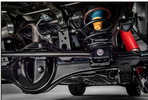
All Tundra models benefit from a new multi-link rear suspension (pictured), chassis and double-wishbone front suspension.
