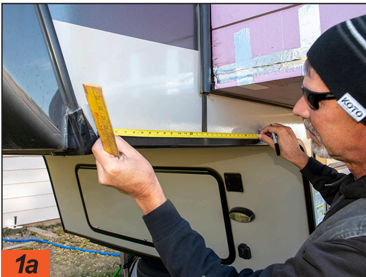
Attaching vinyl skirting to your RV can be done using a variety of methods from hook-and-loop fasteners to twist locks to snaps. The latter is the preferred method by many pro installers like Jorgensen because they are easier to install — and less expensive — than twist locks. Installing the vinyl skirting properly requires laying out the places for the fasteners to attach. He likes to place them about 16 inches apart, and just inches apart around the cargo doors and other corners.
