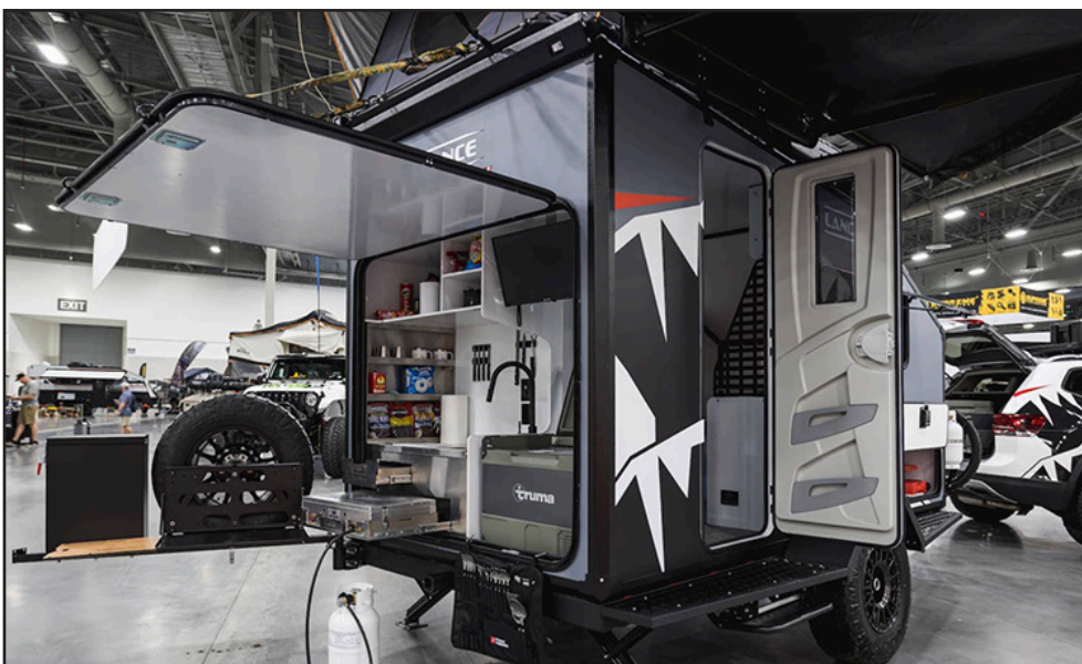
Tucked behind an oversize rear door, the outdoor galley includes a sink, LP-gas-fired griddle, Truma portable refrigeration unit and even a 12-volt DC TV.
