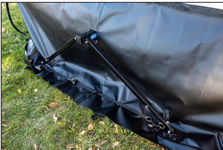
One advantage to having a custom vinyl/canvas skirting installed is the skirts can be tailored to accommodate all types of contours and special needs, like having an opening for the hitch receiver and MORryde rear stabilizer setup on this fifth wheel.
