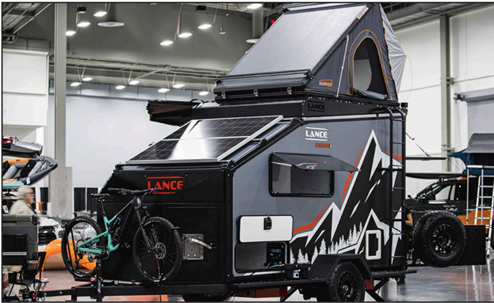
Fully outfitted for off-grid camping, the Lance Enduro boasts a rooftop tent, twin 100-watt solar panels, bike rack and a lot more.
