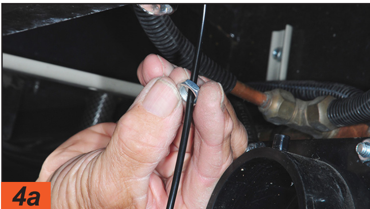
The metal retaining nut is run up the wire to hold the light in place. It can be a little awkward to maneuver the wrench to seat the retaining nut due to the skirt lip angle and surrounding hardware/components. Using a metal nut on aluminum threads could lead to galling, which would make removal difficult. Our worries were short lived, since the thread tolerances are rather sloppy (but still close enough to secure the light without wiggling).
