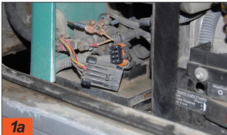
The first step is to pull out the Weather Pack connector to the remote-control unit, which allows remote starting from the switch inside the motorhome. Next, the battery power cable is disconnected.
