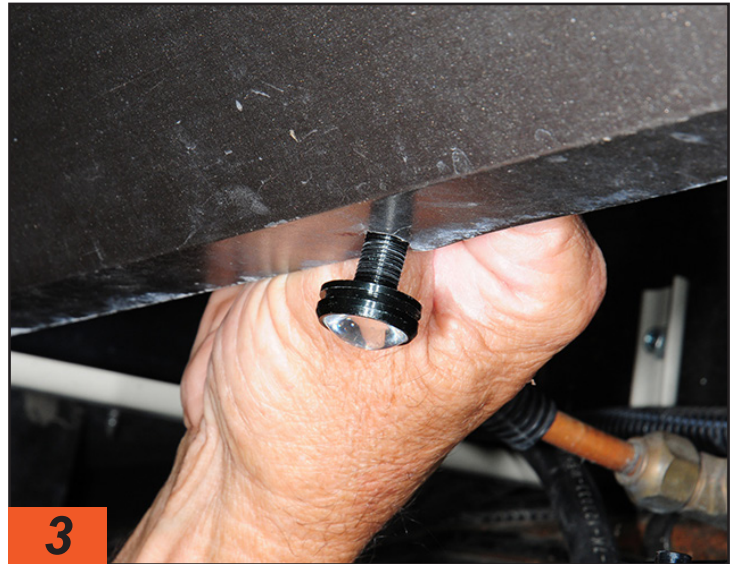
After feeding the wiring pigtail through the hole, the threaded shaft is put into position.
