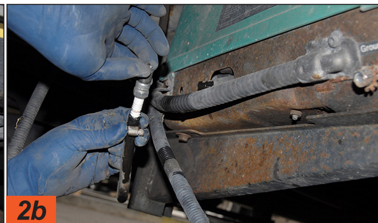
Moving underneath the motorhome, disconnect the ground cable followed by the rubber fuel line. In most cases where the generator is several years old the fuel line will be brittle and difficult to remove, so it will likely be easier to cut it off. The technician used an old spark plug in the line after it was cut to prevent fuel from dripping.
