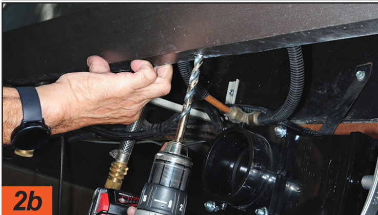
After feeding the wiring pigtail through the hole, the threaded shaft is put into position.
