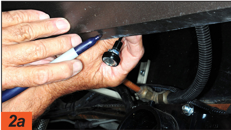
The threaded aluminum alloy shaft is measured with a gauge to determine the right size bit for drilling the hole in the metal skirt
