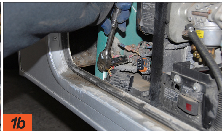
The first step is to pull out the Weather Pack connector to the remote-control unit, which allows remote starting from the switch inside the motorhome. Next, the battery power cable is disconnected.
