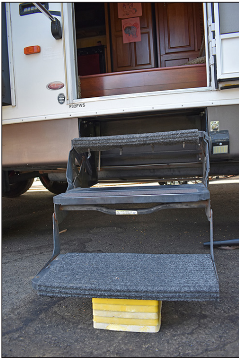
The original pull-out steps were worn out and not capable of supporting occupants without using a wood-block brace for stability. It was an unsafe situation.
