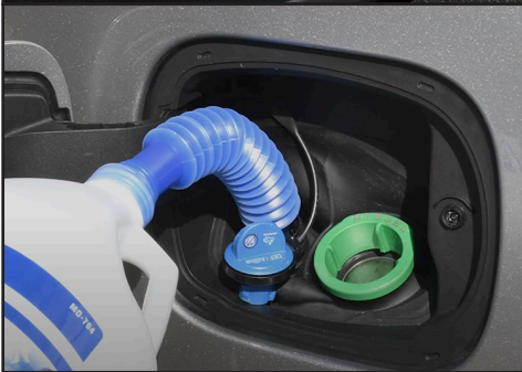
Late-model Ram pickups (2020 Ram 1500 shown here) incorporate a gauge in the instrument cluster to monitor DEF level. The fluid is added to a special reservoir accessed behind the fuel filler door on the pickup.
