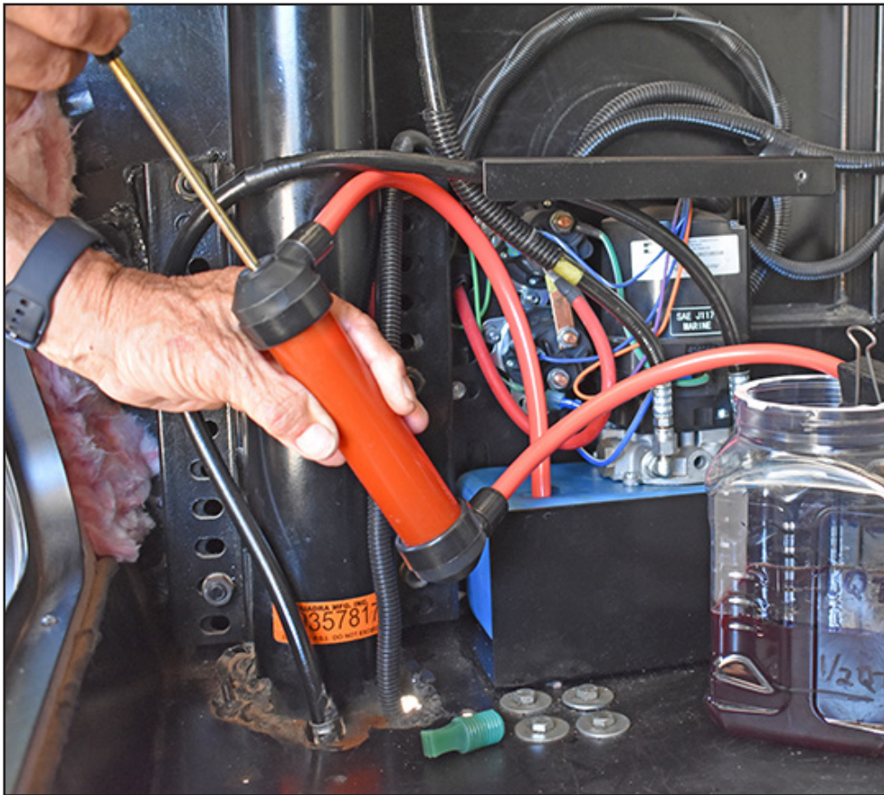
A siphon pump allows fluid from the reservoir to flow into an adjacent container. This pump is easily found online or at auto parts stores. Do not reuse the fluid removed from the reservoir.
