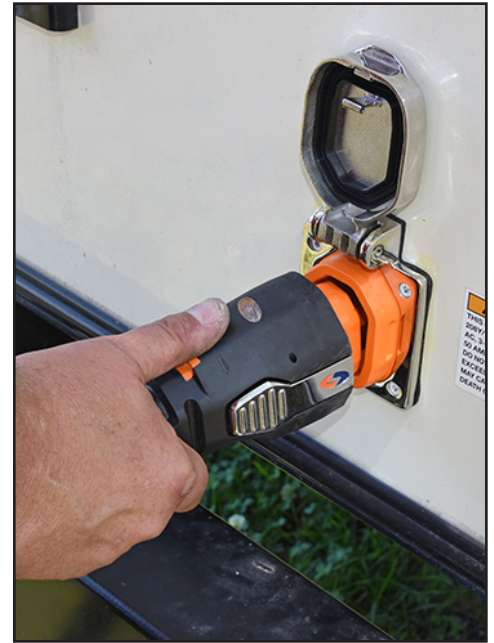
To connect, lift the door, press the plug in until the two side metal latches click into place, then lower the door to lock it onto the plug.
