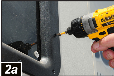
Inner window-frame screws are removed with a screw gun. The inner frame is carefully removed, paying close attention to whether the outer frame and window will release on its own.
