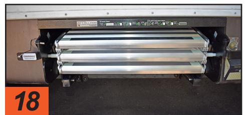
When folded for travel, steps are neatly tucked into the well under the entry door. Only 6 inches of clearance are needed to deploy the steps—perfect for tight storage spaces.
