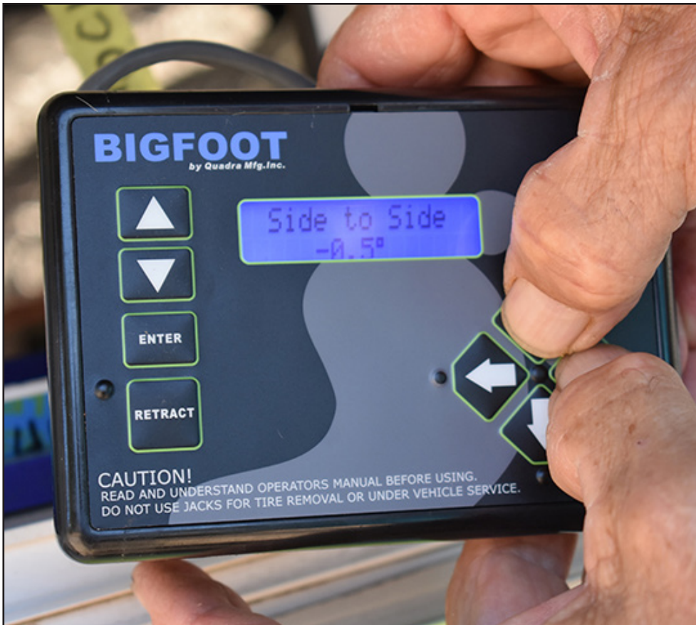
Run the jacks up and down a few times to circulate the additive. It might be necessary to bleed the system again to remove the air bubbles, but that determination might not be immediate.
