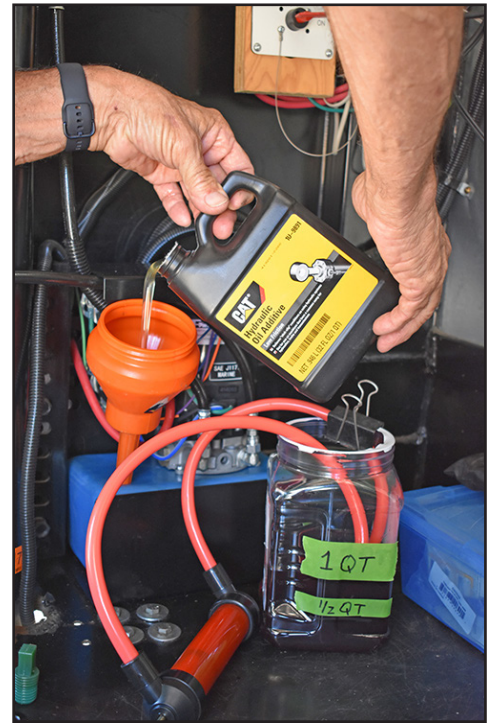
Using a clean funnel, add about half the quart container of Caterpillar Hydraulic Oil Additive to the reservoir. Make sure you removed at least that much fluid from the reservoir first — or, better yet, give yourself some space and remove closer to a quart to make sure the additive does not overflow.
