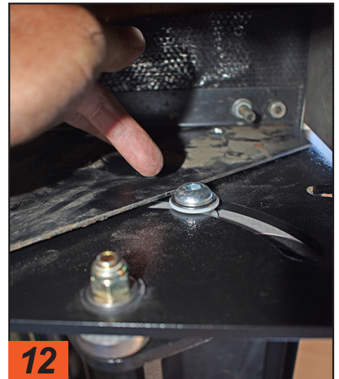
Further inspection revealed that travel for the mechanism was being restricted by the original frame. Here, you can see that the bolt on each side does not have enough travel clearance for retracting the new steps.
