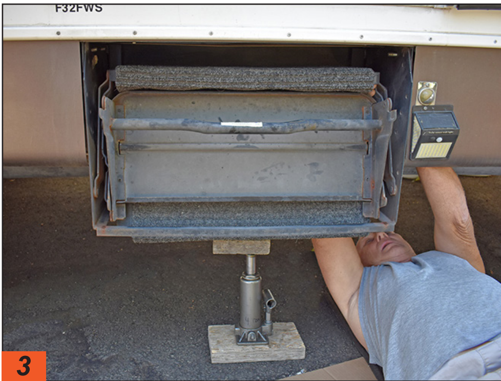
A hydraulic bottle jack and wood block are placed under the bottom step of the original system to ensure safety when removing the bolts.
