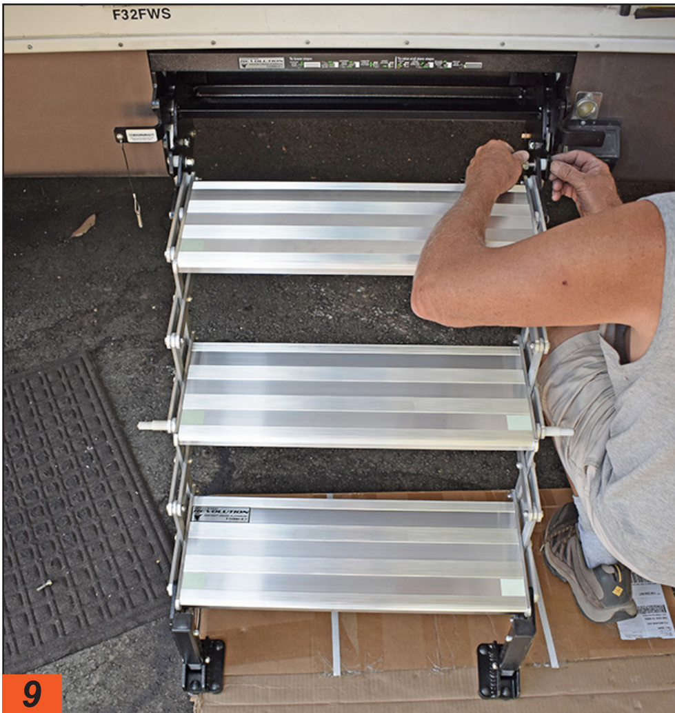
After securing the new frame, the step assembly is aligned properly and reattached.
