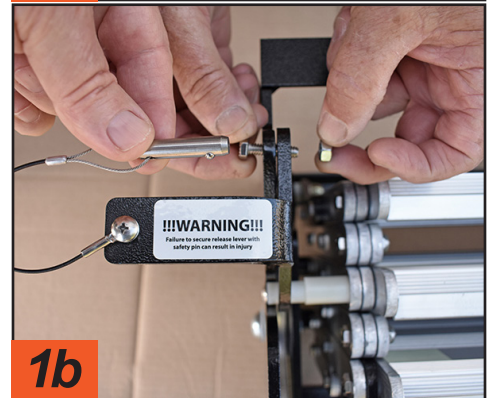
After unboxing, the bolt that secures the steps for shipping is removed and the pin that locks the steps in the stored position is installed. The shipping bolt that was removed after unboxing is installed in the top link permanently.
