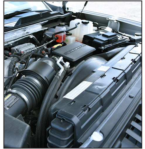
For the 2020 model year, GM offered the 6.6-liter Duramax diesel with an all-new Allison 10-speed automatic transmission that bestowed 3500 series trucks with a towing capability of up to 35,500 pounds — a 52% increase over previous years.
