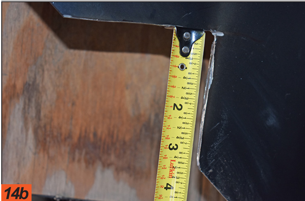
A grinder was used to make the cut. The owners of this particular fifth wheel had to make 3-3/8- x 4-inch cuts in the factory panel.
