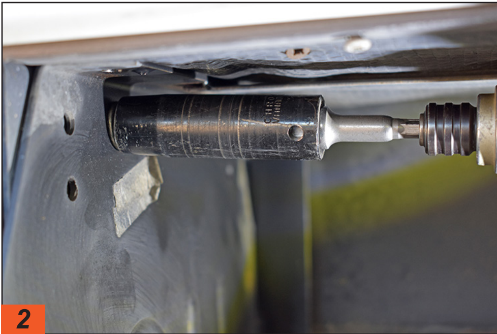
Bolts securing the original steps are removed from the factory side frame panels.
