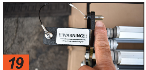
An aforementioned pin prevents the steps from unfolding while in storage/travel mode. RVE
