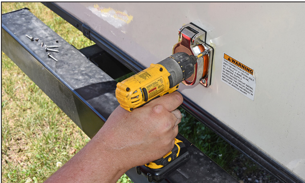
The unit is secured to the wall with user-provided screws. The holes lined up perfectly in this case, but may not always. The old gasket had discolored the fiberglass, but most of the area was covered up by the new receptacle.
