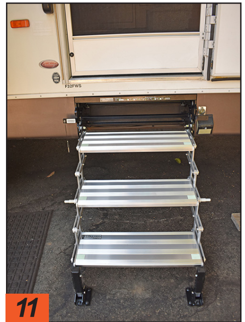
The new steps fit nicely and looked like they were ready for action. Well, not so fast. For some reason, the builders of this fifth wheel strayed somewhat from their tolerances for this model and the step would not retract.
