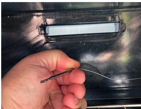
The oven temperature bulb should also be clean. In this case, it was sitting on the floor of the oven; the bracket for the bulb, which goes in the hole in the back, was missing.
