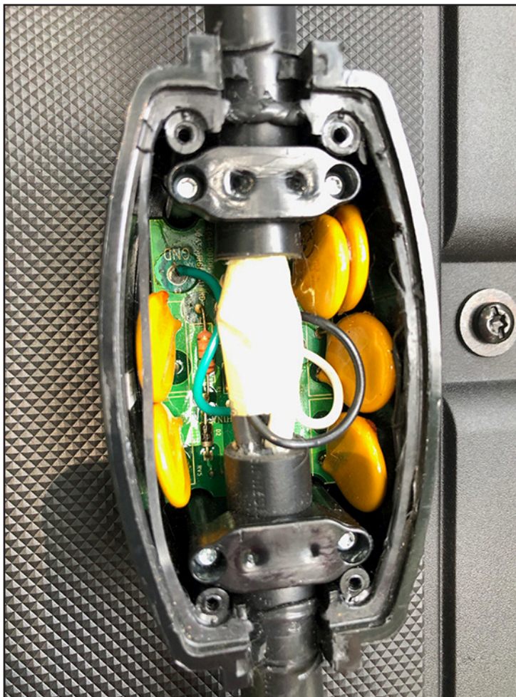
Metal Oxide Varistors (the yellow coin-shaped objects seen here) are the sacrificial elements inside of a surge protector. Each surge event causes some deterioration of the MOVs, but a massive surge could destroy all of them. Without MOVs, destructive energy would be passed on to all the electronics in your RV, causing damage that can cost thousands of dollars. Mike Sokol photo
