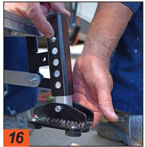
Landing jacks can be adjusted to support steps, even on undulating terrain. This feature makes it unnecessary to carry wood blocks for stabilizing the steps.
