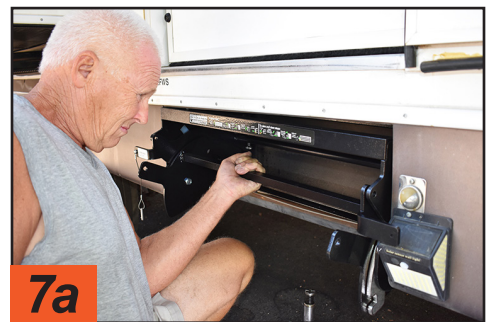
When installing the new steps, the best option is to remove the step assembly from its frame to reduce weight and make it practical for one person to make the swap.
