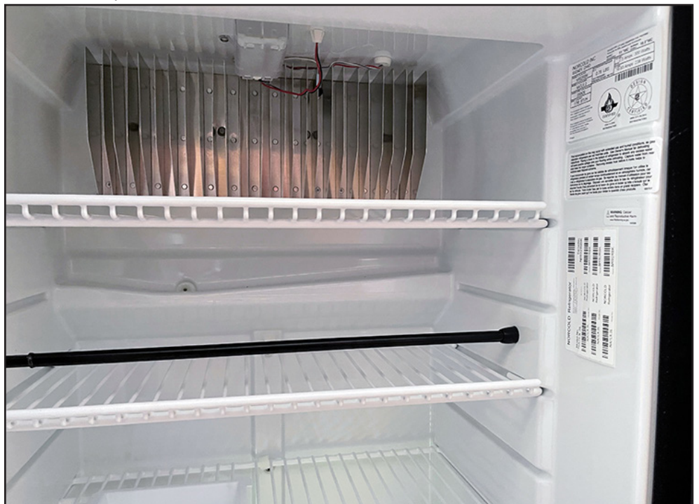
The inside of the fresh food compartment has the cooling fins on the upper rear. The thermistor, which reads the temperature in the refrigerator, is clipped to a fin in the middle on this model. If your unit isn't staying cold, check that it is attached correctly. It can detach — which will upset the cooling capability of the refrigerator. Under the fins is a molded-in condensate catcher, which drains to the small hose connection in the rear.
