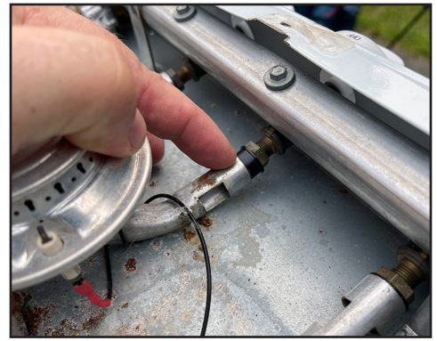
If you remove the burners for cleaning, don't lose the burner bushing! It slides off the valve easily.
