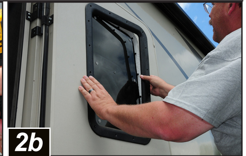
Inner window-frame screws are removed with a screw gun. The inner frame is carefully removed, paying close attention to whether the outer frame and window will release on its own.
