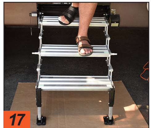
The Torklift steps are very comfortable to negotiate. Space between the door landing and first step is lower than the factory counterpart, and the 7.5-inch rise height between steps makes it easier to enter or exit the trailer.
