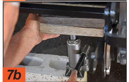
The new frame, minus the step assembly, is positioned into the step well below the entry door. A bottle jack, wood block and brick were called into service to stabilize the structure for proper line up.
