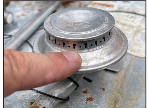
If you have a big boil-over, you might get the ports full of...whatever you're cooking. Remove the burner and soak in hot soapy water and lightly scrub with a stiff bristle brush to clean, being careful not to damage the jets.
