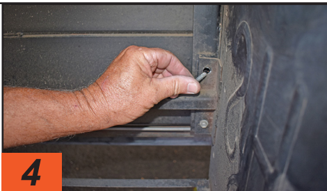
Rear bolts in the original step frame were also removed — a procedure that may not be required on other model fifth wheels. These positions do not apply when installing the new step.
