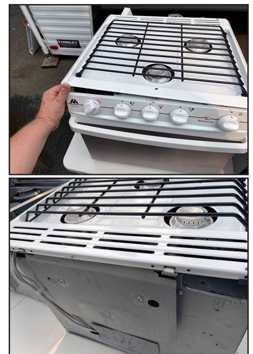
Some ranges have a deck that lifts straight up. This Atwood deck has to be slid straight back to unlatch it, then lifted to release the spring catches for the deck lid.
