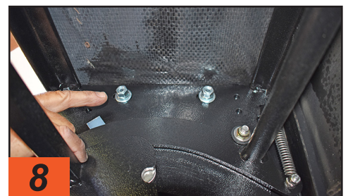
New bolts are installed through the Torklift frame and into the steel step-well panels.
