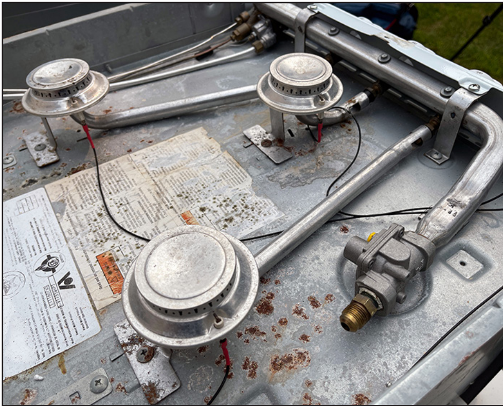
If you remove the burners for cleaning, don't lose the burner bushing! It slides off the valve easily.
