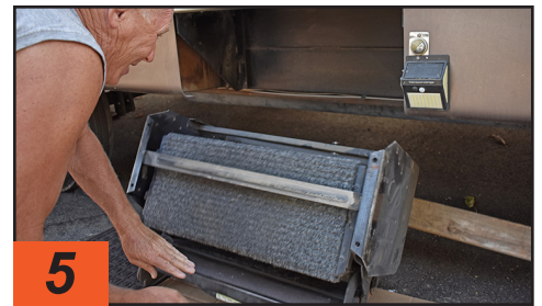
Once all the bolts were removed, the factory steps are removed from the fifth wheel and discarded.
