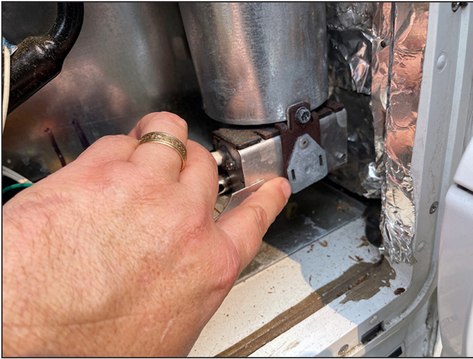
The Norcold has a swinging burner door, which provides easy sighting of the flame and burner. A severely dirty or corroded burner or a pile of rust will require the fridge be pulled out and the burner, chimney and baffle inspected and serviced by a factory-trained service technician or certified RV technician.
