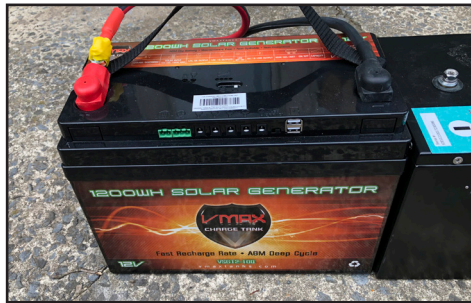
Next, let's take a look at a VMAX 1200WH (actually 100 amp-hour) AGM battery. Note that this battery includes an on-board solar panel charger, which is very handy for upgrades where you
