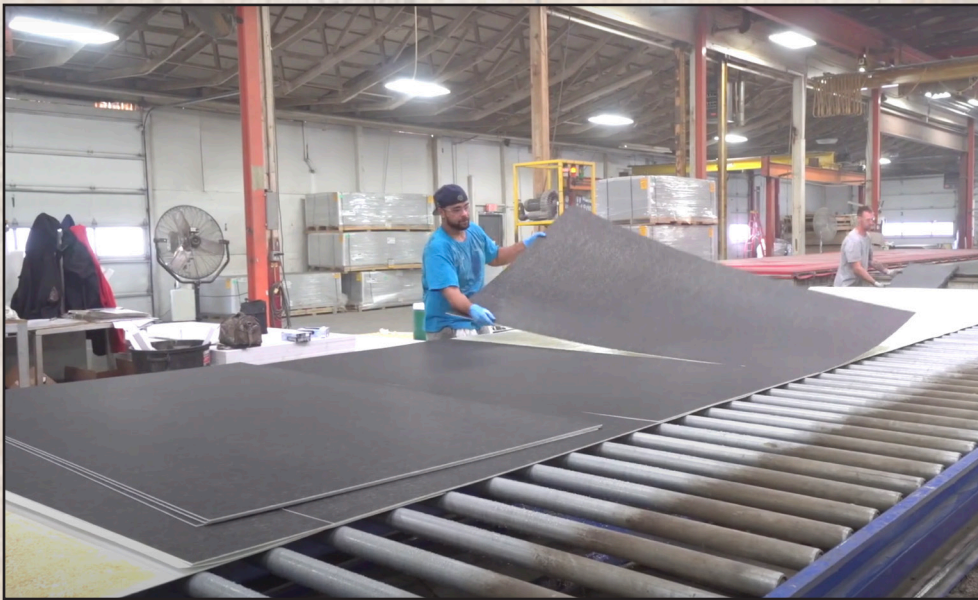
Workers at Azdel's Lynchburg, Virginia, manufacturing facility prepare sheets of the composite for use in RV construction.
