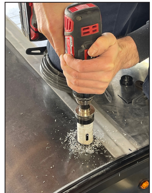
A hole will need to be drilled in the roof to route cables for the solar array. This needs to be planned carefully. In this instance, because of the trailer design, there was one spot to cleanly run the cables, and we still hit structure underneath — but just slightly.
