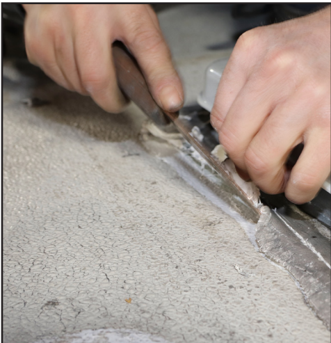
Carefully cut and separate the skylight from the sealant on the roof. It’s okay to scrape on aluminum and fiberglass roofs, but don’t do it on a membrane roof. A heat gun used carefully can help to soften the sealant. Use a flat tool to carefully pry up and remove the skylight, working your way around. A long plastic pry tool should be used on membrane roofs to avoid cutting the membrane. If you do happen to cut it, don’t sweat it. EternaBond is your friend!
