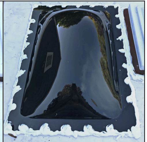
The new skylight was pre-drilled for screws. One-inch putty tape was applied around the screw line on the underside of the flange, then the skylight dome was aligned carefully with the opening and screwed down. It’s best to have someone in the RV to eyeball the skylight alignment in the roof opening. Dacor self-leveling sealant, appropriate for the roof, was then applied.
