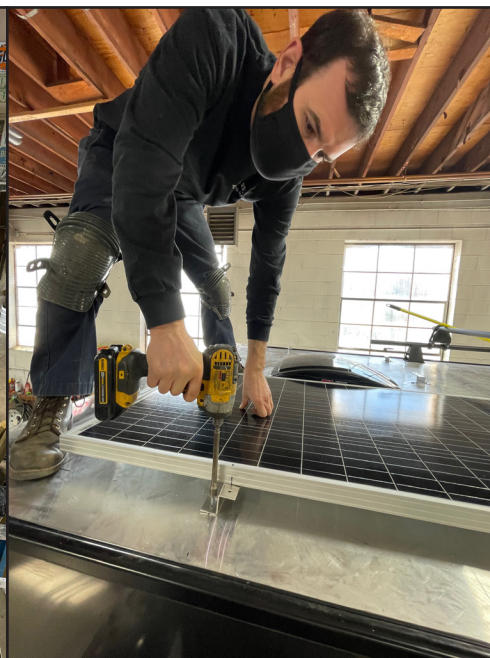
It’s important to find structure in the roof to screw down the panels. Turner marked and measured the location of the roof structure, figured out the best alignment of the panels, lined up the brackets, marked and drilled the panels, test fit them to the panels, removed the brackets, screwed them to the roof using putty tape and sealer, then mounted the panels to the brackets with modified hardware to make them easier to attach.
