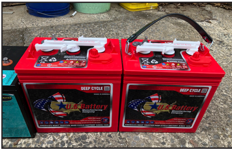
First up is a pair of US Battery US2200XC2 6-volt FLA batteries rated
