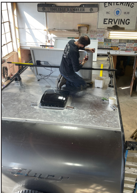
It’s important to find structure in the roof to screw down the panels. Turner marked and measured the location of the roof structure, figured out the best alignment of the panels, lined up the brackets, marked and drilled the panels, test fit them to the panels, removed the brackets, screwed them to the roof using putty tape and sealer, then mounted the panels to the brackets with modified hardware to make them easier to attach.
