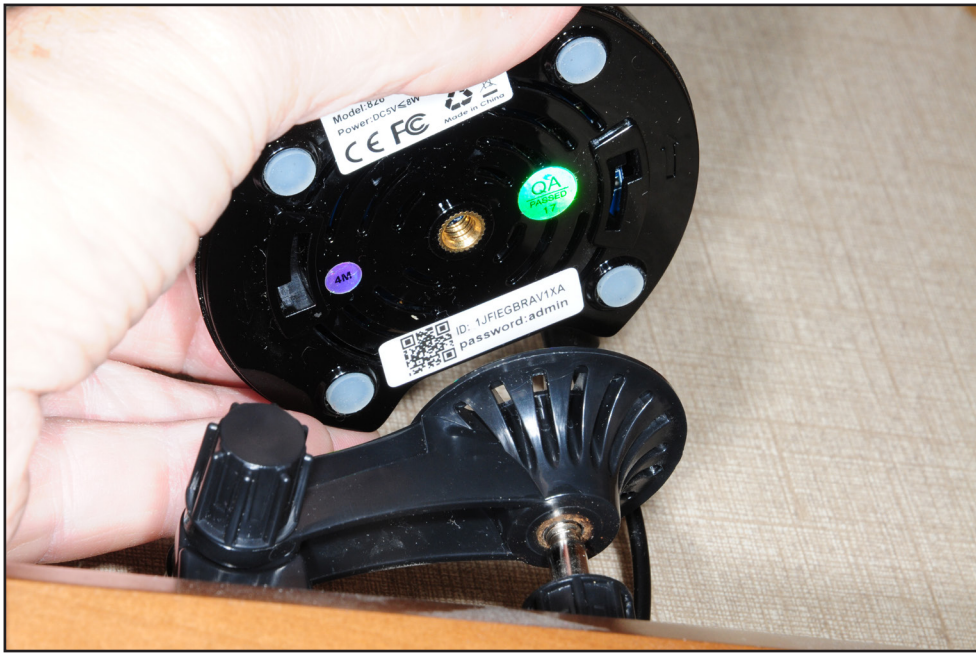
The plastic bracket that comes with the camera was attached to a flat spot behind the decorative molding using two wood screws. Once in place, the camera can be removed for travel by loosening the hold-down bolt with the knurled knob.
